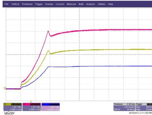
Top, 5V output, 1V/div; Middle, 3.3V output, 1V/div; Bottom, 10V output, 5V/div
