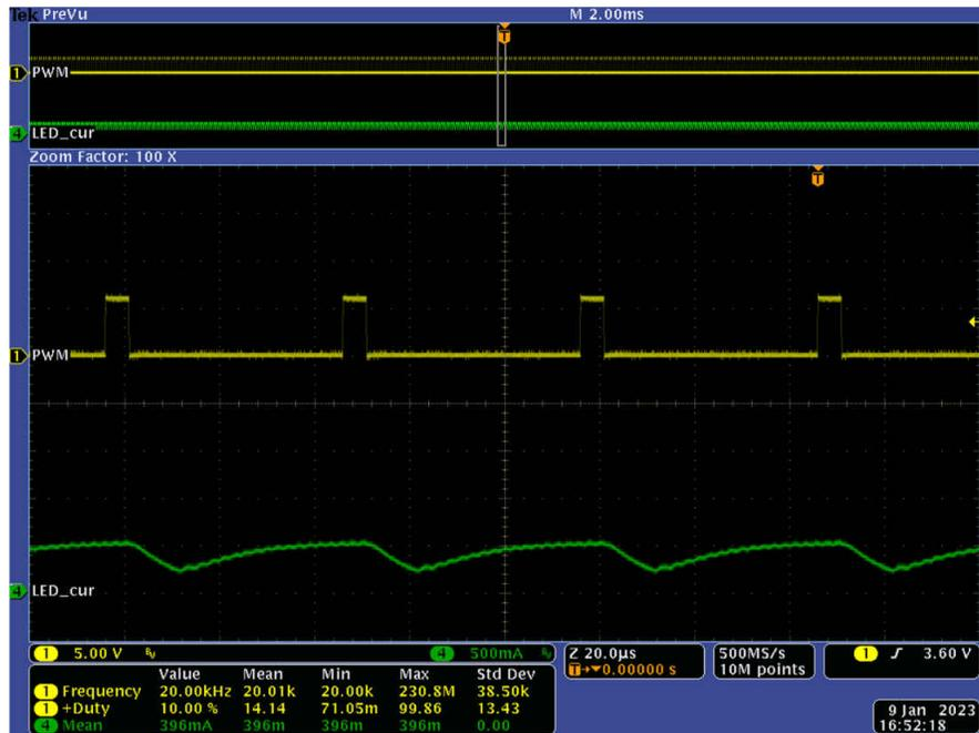
Figure 5-11. Waveforms at 10% Duty Cycle, 20 kHz Hybrid Dimming
