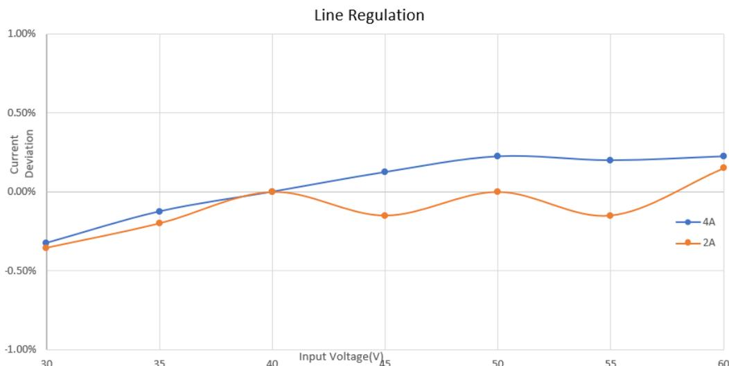
Figure 5-3. LED Current Deviation vs. Input Voltage
