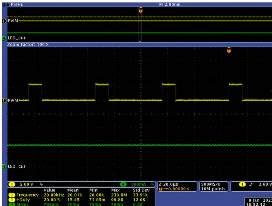
Figure 5-12. Waveforms at 20% Duty Cycle, 20 kHz Hybrid Dimming
