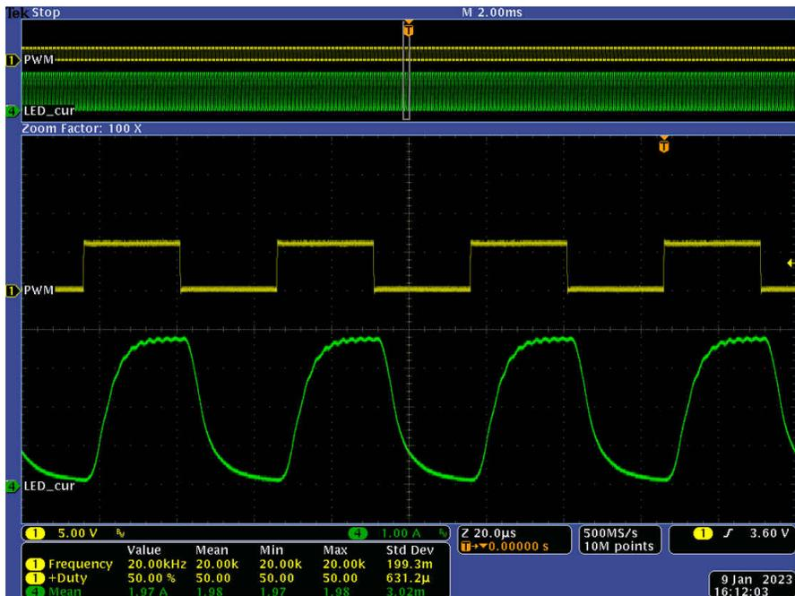
Figure 5-8. Waveforms at 50% Duty Cycle, 20 kHz PWM Dimming
