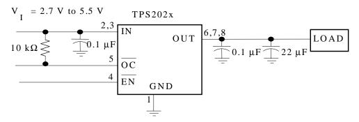
Figure 1. Typical Implementation With the TPS202X
