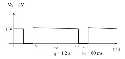
Figure 2. Over Current Protection and Thermal Shutdown for 3.3- $\Omega$  Load (TPS2020)
