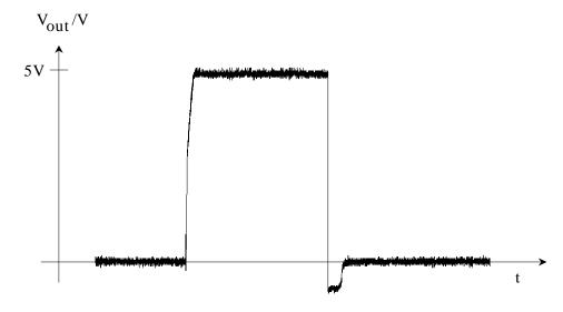
Figure 3. Output Voltage of a TPS2020 Driving a 5-V Relay
