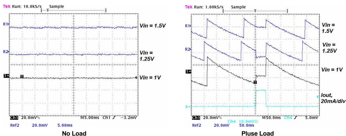
**Figure 10. Output Ripple Voltage During PFM-Mode Operation With 22- $\mu\text{H}$  Inductance,  $2 \times 4.7\text{-}\mu\text{F} + 120\text{-}\mu\text{F}$  (C5) Output Capacitor**
