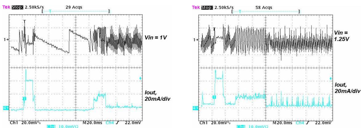
**Figure 1. High Ripple Voltage Causes the Bluetooth Chipset to Draw Excessive Current During Sniff-Mode Operation**
