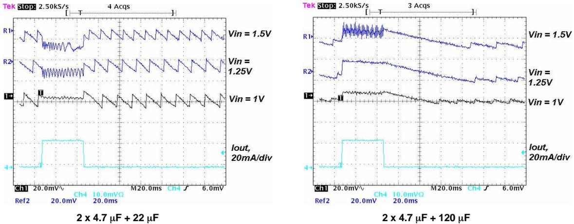
Figure 11. Output Ripple Voltage During PFM-Mode Operation With 1-nF Feedforward Capacitor (Cff), 4.7- $\mu$ H Inductor, and With Different Output Capacitors
