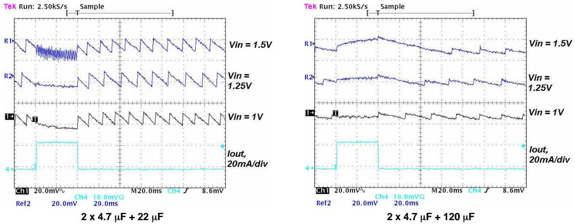
**Figure 16. Output Ripple Voltage During PFM-Mode Operation With 100-nF Feedforward Capacitor (Cff), 10-µH Inductor, and With Different Output Capacitors**
