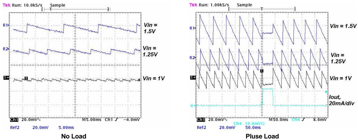
Figure 7. Output Ripple Voltage During PFM-Mode Operation With 10- $\mu$ H Inductance, 2  $\times$  4.7- $\mu$ F + Additional 22- $\mu$ F (C5) Output Capacitor
