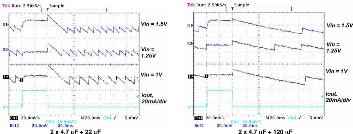
Figure 18. Output Ripple Voltage During PFM-Mode Operation With 10-nF Feedforward Capacitor (Cff), 22-μH Inductor, and With Different Output Capacitors
