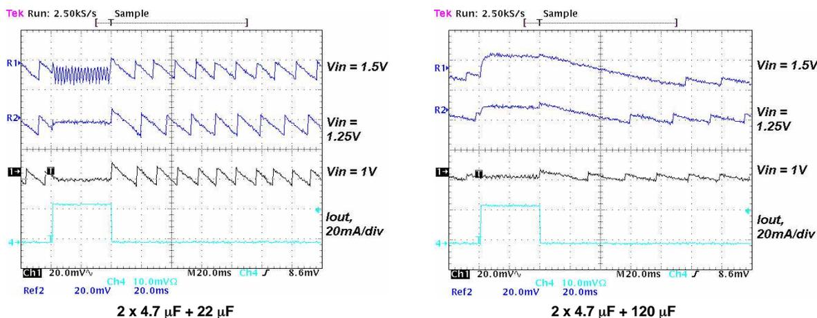
Figure 15. Output Ripple Voltage During PFM-Mode Operation With 10-nF Feedforward Capacitor ( $C_{ff}$ ), 10- $\mu\text{H}$  Inductor, and With Different Output Capacitors
