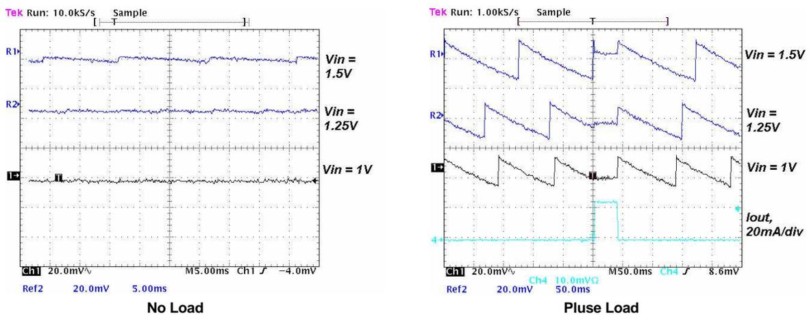
Figure 8. Output Ripple Voltage During PFM-Mode Operation With 10- $\mu$ H Inductance, 2  $\times$  4.7- $\mu$ F + Additional 120- $\mu$ F(C5) Output Capacitor
