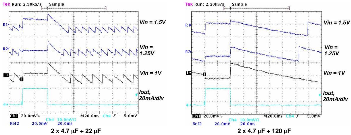
**Figure 17. Output Ripple Voltage During PFM-Mode Operation With 1-nF Feedforward Capacitor (Cff), 22-µH Inductor, and With Different Output Capacitors**
