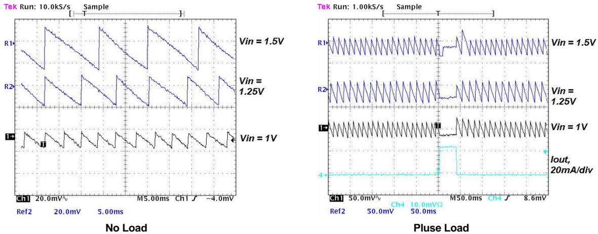
Figure 6. Output Ripple Voltage During PFM-Mode Operation With 10- $\mu$ H Inductance, 2  $\times$  4.7- $\mu$ F Output Capacitor (Note the change of voltage scale on the right to accommodate the waveforms.)
