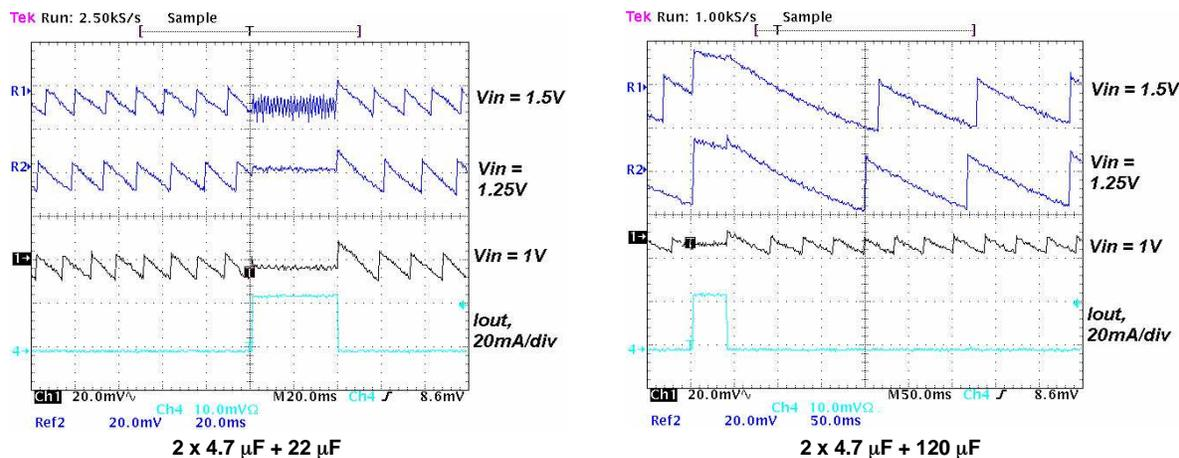
Figure 14. Output Ripple Voltage During PFM-Mode Operation With 1-nF Feedforward Capacitor ( $C_{ff}$ ), 10- $\mu\text{H}$  Inductor, and With Different Output Capacitors
