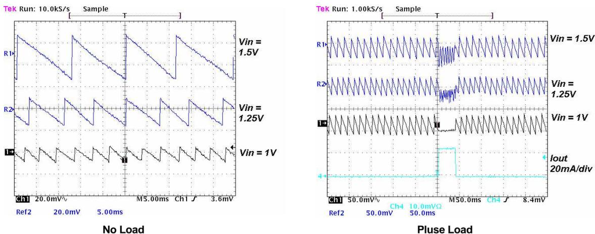
Figure 3. Output Ripple Voltage During PFM-Mode Operation With Original EVM Setup of 4.7- $\mu\text{H}$  Inductor and  $2 \times 4.7\text{-}\mu\text{F}$  Output Capacitors (Note the change of voltage scale on the right to accommodate the waveforms.)
