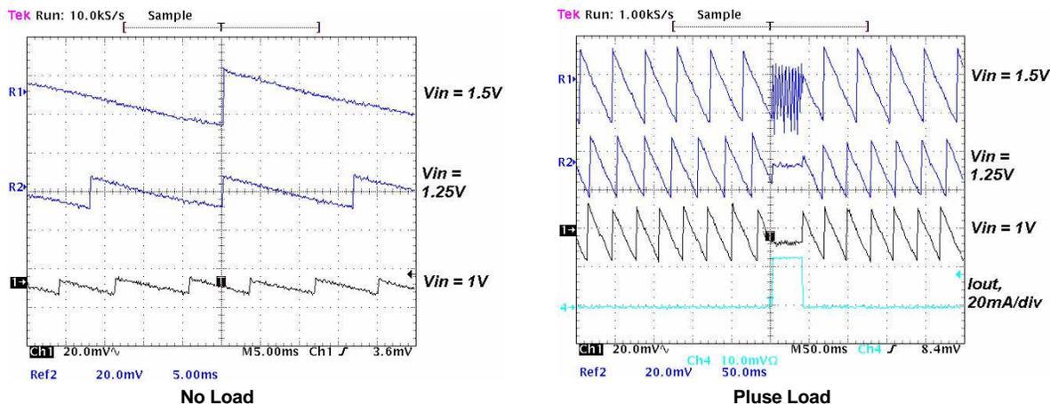
Figure 4. Output Ripple Voltage During PFM-Mode Operation With Additional 22- $\mu$ F Output Capacitor (C5)
