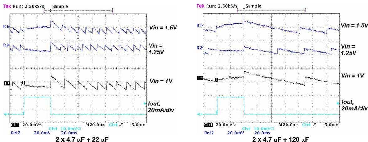
Figure 19. Output Ripple Voltage During PFM-Mode Operation With 100-nF Feedforward Capacitor (Cff), 22-μH Inductor, and With Different Output Capacitors
