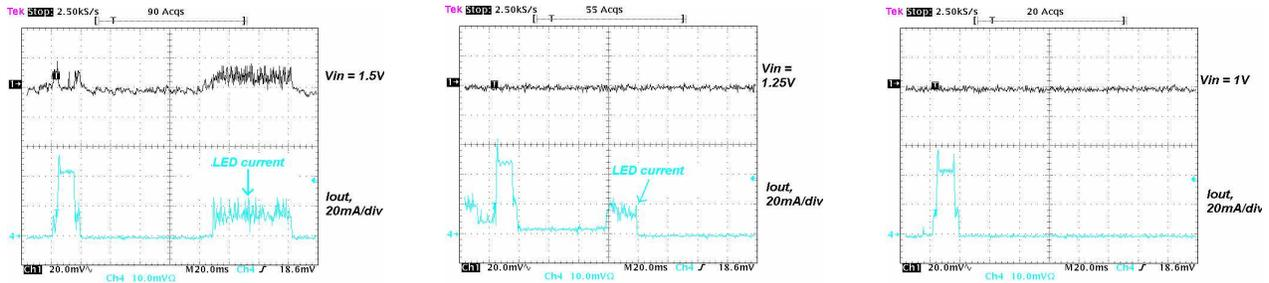
Figure 20. Output Ripple Voltage and Current Waveform From TPS61070 During Sniff-Mode Operation of Bluetooth Headset With 1-nF Feedforward Capacitor (C<sub>ff</sub>) and With 2 × 22-μF Output Capacitors
