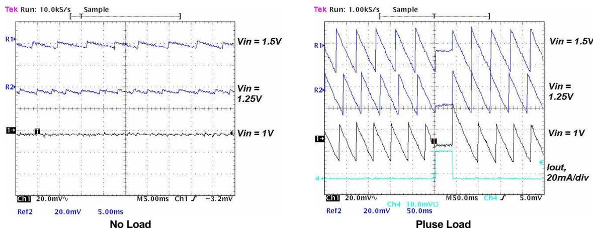
**Figure 9. Output Ripple Voltage During PFM-Mode Operation With 22- $\mu\text{H}$  Inductance,  $2 \times 4.7\text{-}\mu\text{F} + 22\text{-}\mu\text{F}$  (C5) Output Capacitor**
