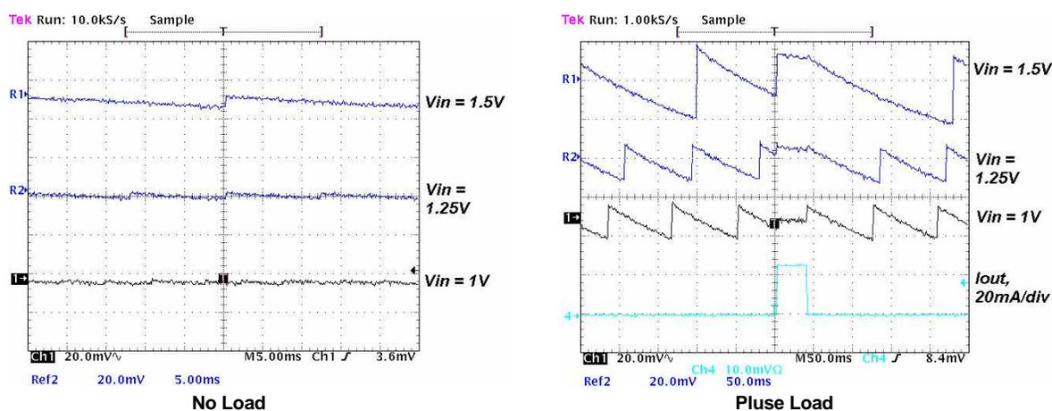
Figure 5. Output Ripple Voltage During PFM-Mode Operation With Additional 120- $\mu$ F Output Capacitor (C5)
