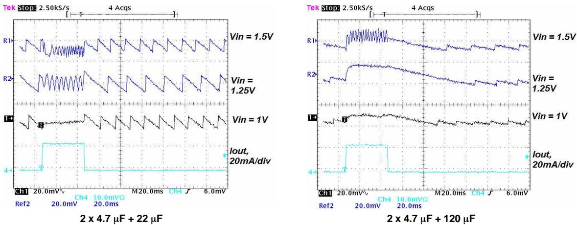
Figure 12. Output Ripple Voltage During PFM-Mode Operation With 10-nF Feedforward Capacitor (Cff), 4.7- $\mu$ H Inductor, and With Different Output Capacitors
