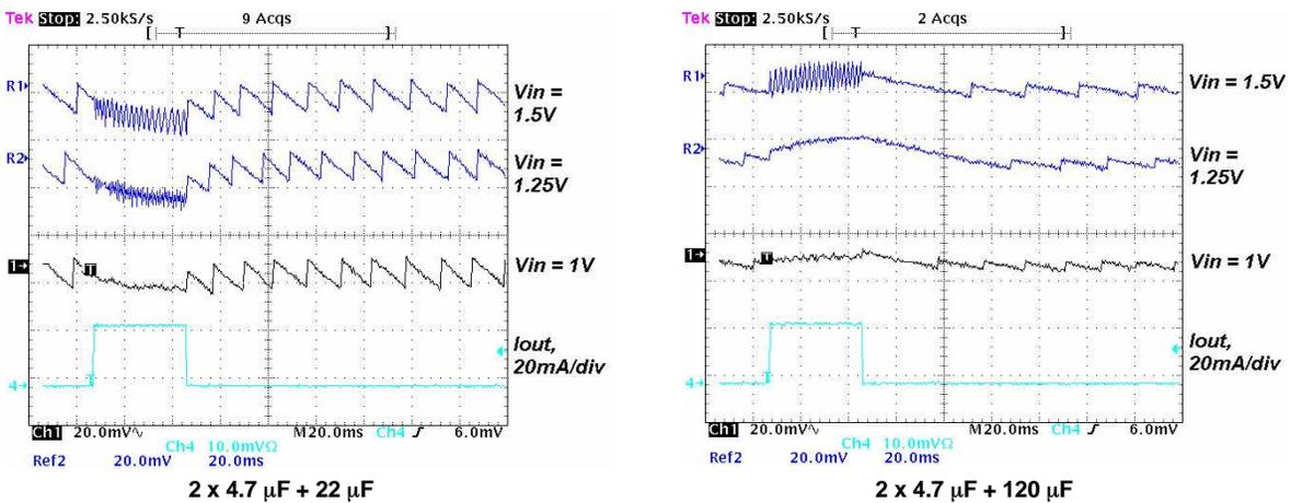
Figure 13. Output Ripple Voltage During PFM-Mode Operation With 100-nF Feedforward Capacitor (Cff), 4.7- $\mu$ H Inductor, and With Different Output Capacitors
