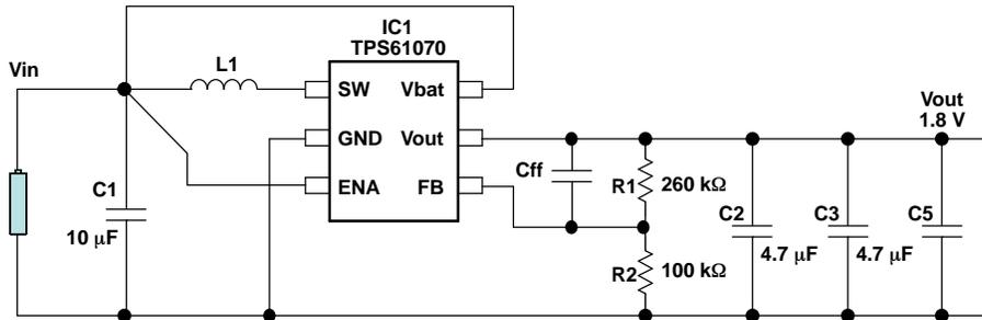
Figure 2. Test Circuit of TPS61070 for Single-Cell Alkaline Battery to 1.8-V Output
