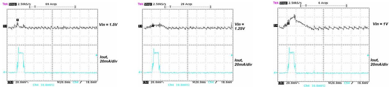
Figure 21. Output Ripple Voltage and Current Waveform From TPS61070 During Sniff-Mode Operation of Bluetooth Headset With 10-nF Feedforward Capacitor (C<sub>ff</sub>) and With 2 × 22-μF Output Capacitors
