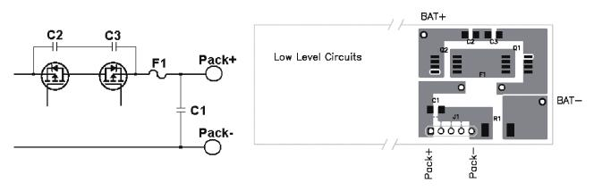
Figure 3. Use Wide Copper Traces to Lower the Inductance of Bypass Capacitors C1, C2, C3
