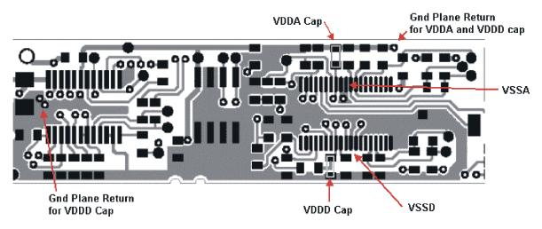
Figure 1. Bad Example of Decoupling Capacitor Placement and Routing
