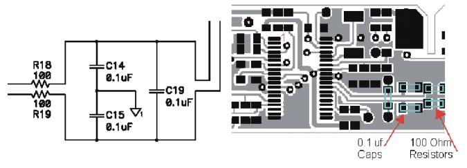
Figure 7. Differential Filter Components With Symmetrical Layout
