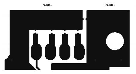
Figure 8. Recommended Spark Gap Pattern Helps Protect Communication Lines From ESD
