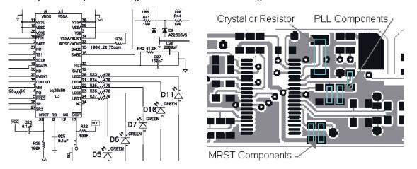
Figure 2. Minimize Length and Loop Area for These Critical Components to Reduce Noise Pickup
