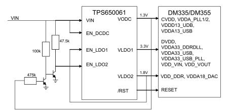
Figure 1. TPS650061 and DM335/55 Simplified Block Diagram
