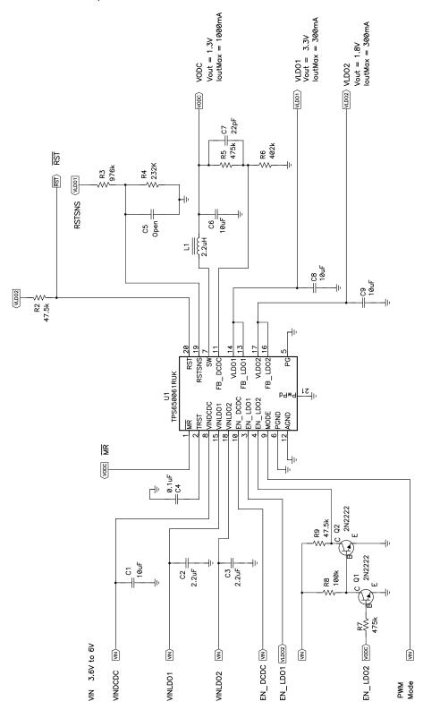
Figure 2. TPS650061 Schematic Diagram
