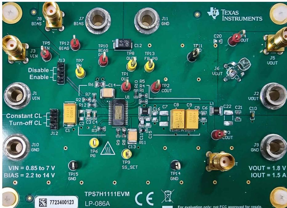
Figure 3-2. TPS7H1111-SEP SEE Test Board Top View
