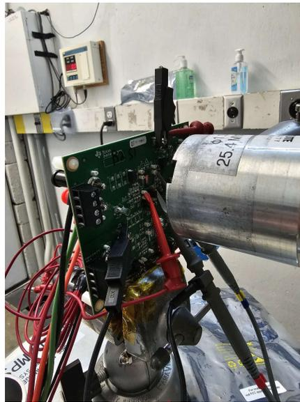
**Figure 4-1. Photograph of the TPS7H2201-SEP Evaluation Board Mounted in Front of the Heavy-Ion Beam Exit Port at the Texas A&M Cyclotron**
