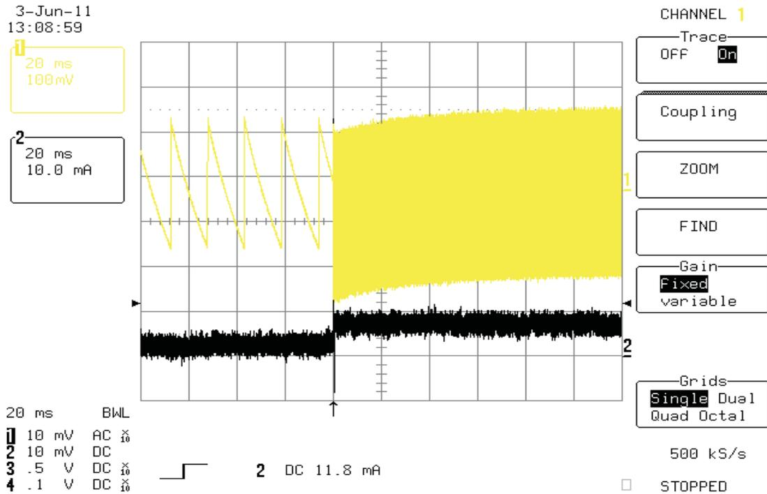
Figure 9. Load Transient, Boost : Vbat = 3.6 V with 0 mA to 5 mA Transient, Constant 15 mA Load on LDO. CH3 Bstout CH4 IBOUST
