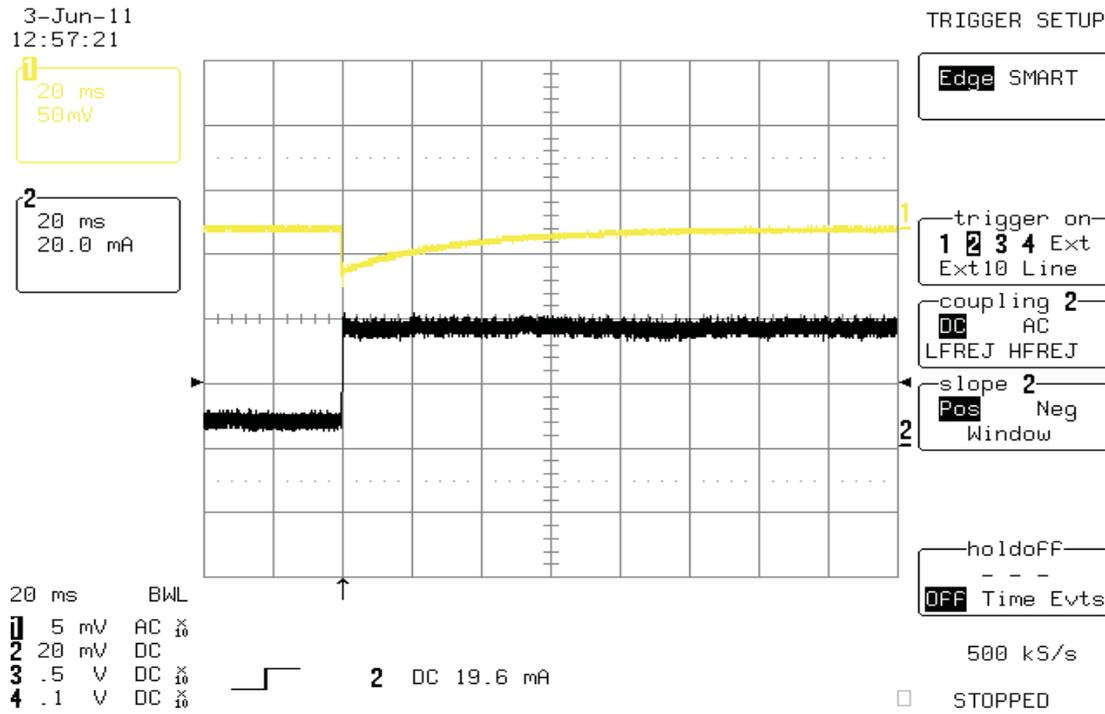
Figure 11. Load Transient, LDO : Vbat = 3.6 V with 0 mA to 30 mA Transient.
