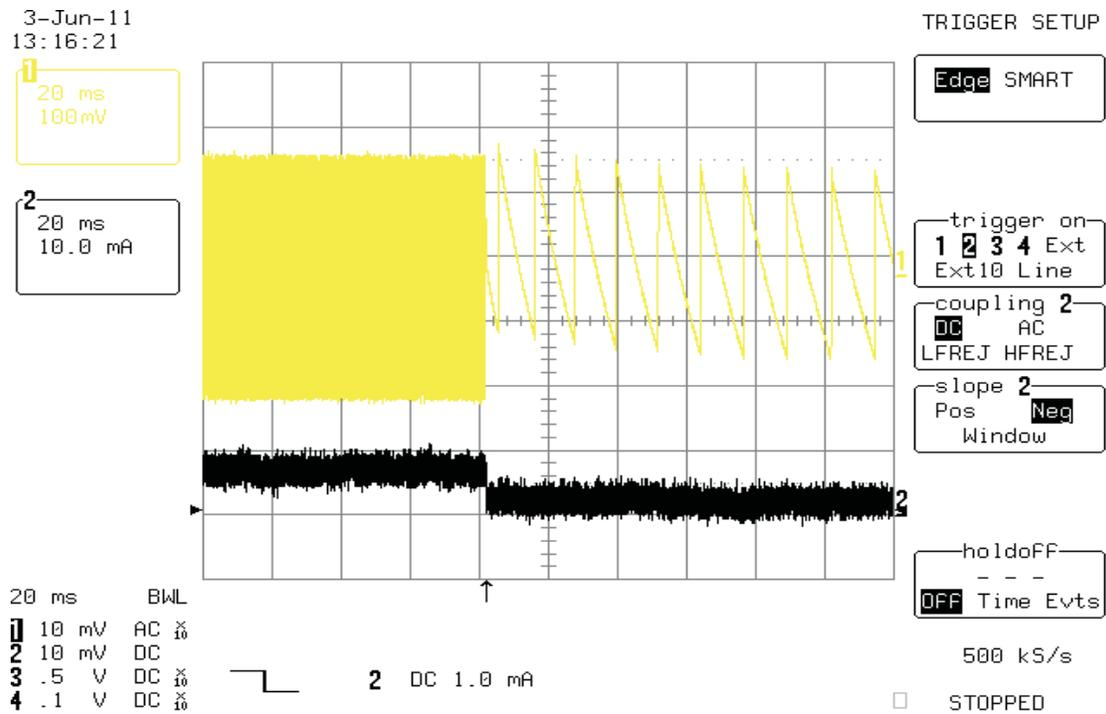
Figure 10. Load Transient, Boost : Vbat = 3.6 V with 5 mA to 0mA Transient, Constant 15 mA Load on LDO. CH3 Bstout CH4 IBOUST
