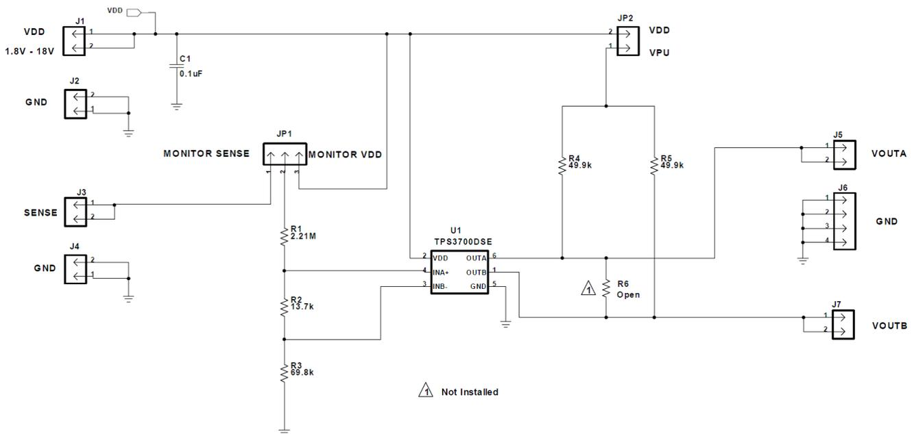
Figure 6. TPS3700EVM-202 Schematic
