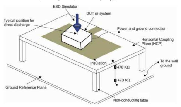
Figure 3. System Level ESD Test Setup
