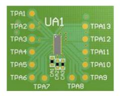
Figure 2. 1 of 3 TPD12S520RMN for IEC-61000-4-2 Tests
