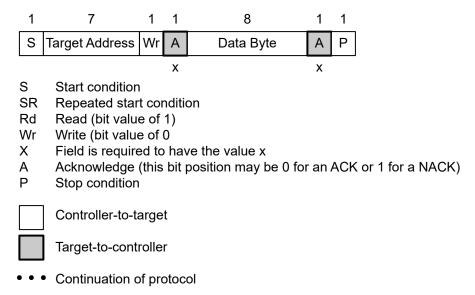
Figure 1-1. I2C Read/Write Protocol Key
