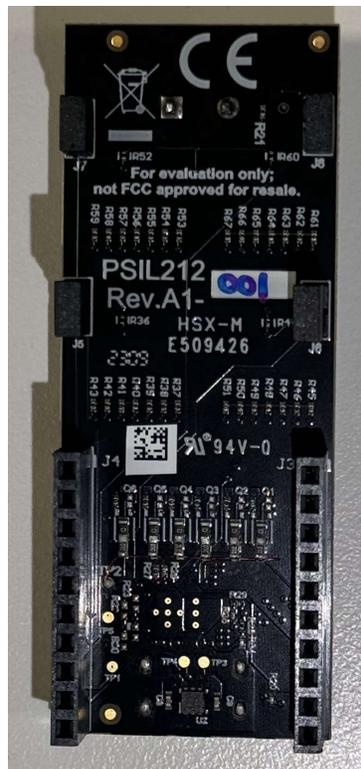
**Figure 2-1. TPS25730EVM Bottom View of the Jumper Locations**
