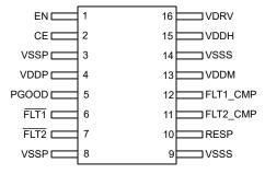
Figure 2-2. TPSI311x-Q1 DVX Package 16-Pin SSOP Top View
