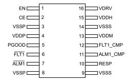
Figure 2-1. TPSI310x-Q1 DVX Package 16-Pin SSOP Top View
