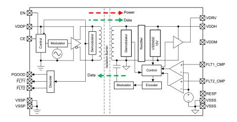
Figure 1-3. TPSI311x-Q1 Functional Block Diagram
