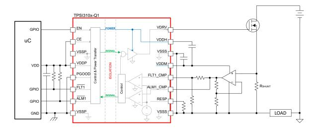
Figure 1-1. TPSI3100-Q1 Simplified Schematic
