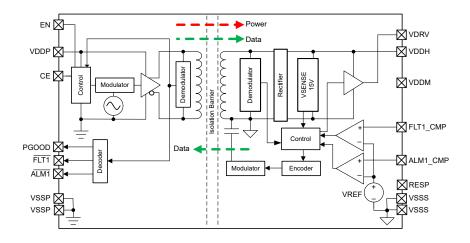
Figure 1-2. TPSI310x-Q1 Functional Block Diagram
