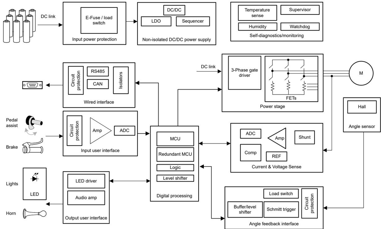
**Figure 4. E-Bike Block Diagram**
