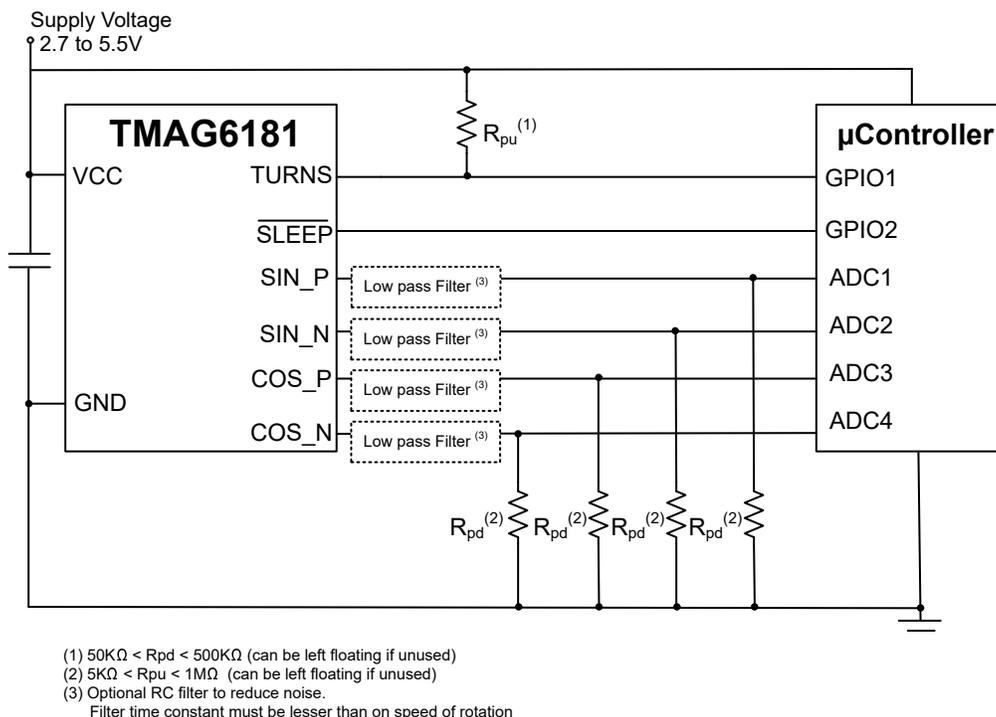
**Figure 3. The TMAG6181-Q1 in Single-Ended Output Mode**
