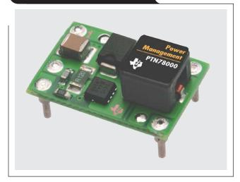
Wide-input power modules typically integrate input and output capacitors. However, additional input or output capacitors may be needed on the host PC board if there are long input lines to the module coupled with high di/dt requirements or if very low-noise outputs are required.
