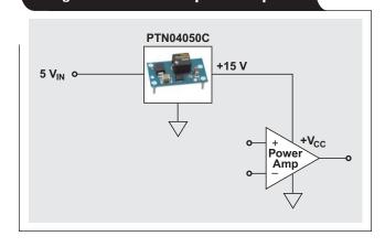
ability to operate from 3.3- or 5-V bus systems, a boost module can be used together with a positive step-down module to create plus and minus voltage rails required by many analog ICs such as op amps and data converters.
