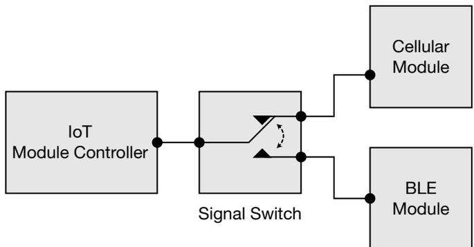
Figure 3. IoT node with two communication modules.
