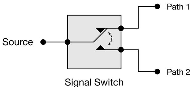
Figure 2. Block diagram of a simple signal switch.
