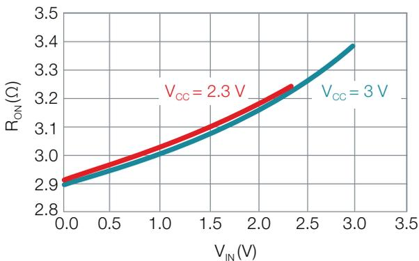
**Figure 5.** Example graphs of  $R_{ON}$  spec vs  $V_{IN}$ .
