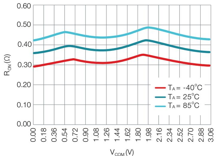
For IoT applications that are very sensitive to  $R_{ON}$  shifts, select switches where the  $R_{ON}$  does not change drastically over the operating voltage range expected for that application. Do consider lower  $R_{ON}$  switches with relatively flat  $R_{ON}$  over voltage and temperature when selecting devices for IoT.
