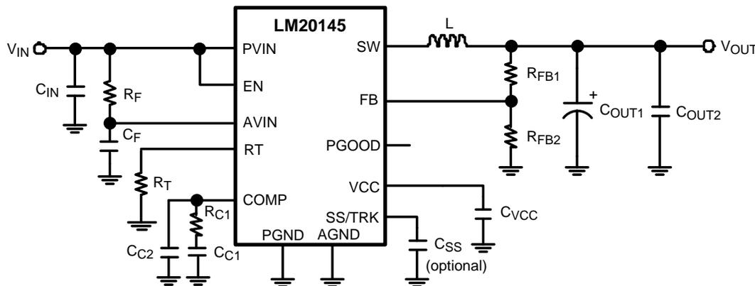
**Figure 5. 1.2V Output Solution Optimized for Load Transients**
