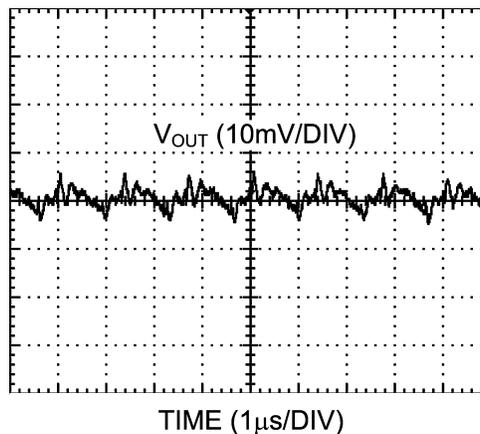
**Figure 7. Output Voltage Ripple**
