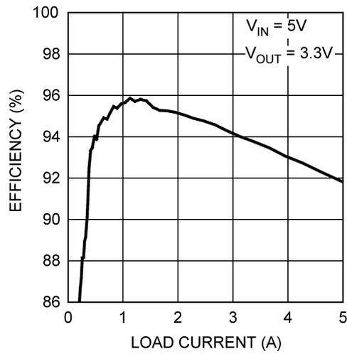
**Figure 2. Efficiency vs  $I_{OUT}$**
