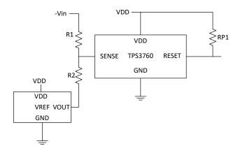
Device shown: TPS3760A012DYYR adjustable threshold variant
