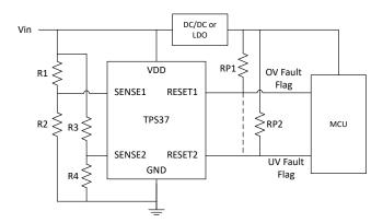
Device shown: TPS37A010122DSKR adjustable threshold variant
