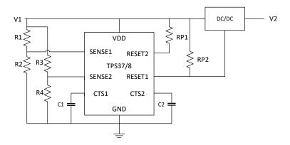
**Device shown:** TPS37A010122DSKR adjustable threshold variant or TPS38A010122DSKRQ1 adjustable
