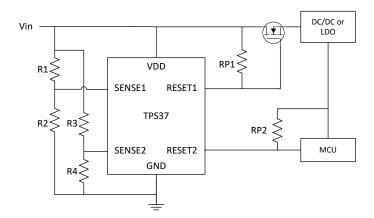
Device shown: TPS37A010122DSKR adjustable threshold variant
