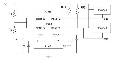
Device shown: TPS38A010122DSKRQ1 adjustable threshold variant
