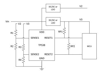
Device shown: TPS38A010122DSKRQ1 adjustable threshold variant
