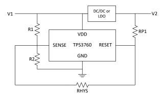
Device shown: TPS3760A012DYYR adjustable threshold variant
