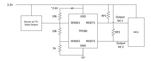
Device shown: TPS38J010155DSKRQ1 adjustable threshold variant
