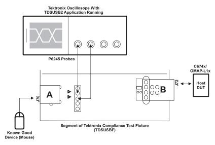
Figure 24. Equipment Setup for Low-Speed Downstream Host Signal Quality Testing
