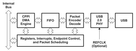
Figure 1. USB Functional Block Diagram
