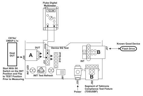
Figure 20. Equipment Setup for Downstream Test J/K, SEO\_NAK
