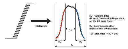
Figure 7. Random Jitter/Deterministic Jitter/Total Jitter
