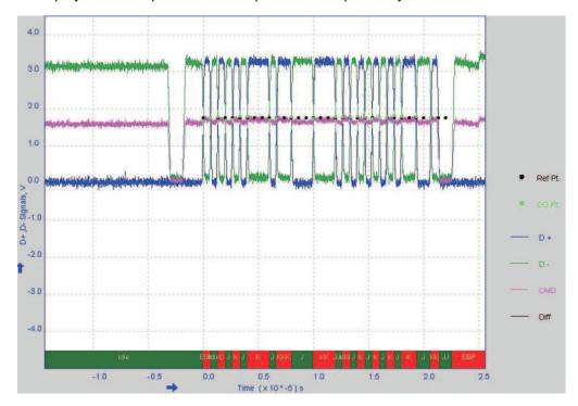
Figure 25. Low-Speed Waveform Plot
