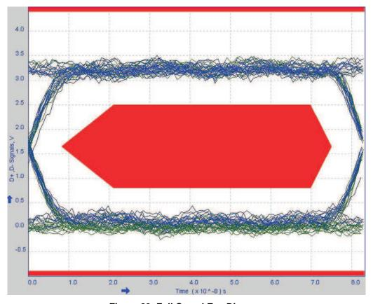
Figure 23. Full-Speed Eye Diagram
