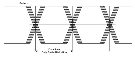
Figure 6. Duty Cycle Distortion (DCD)
