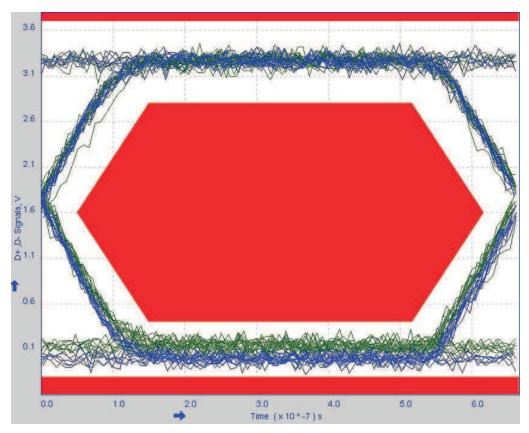
Figure 26. Low-Speed Eye Diagram
