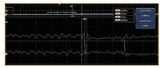
Figure 15. Downstream Chirp Response Time
