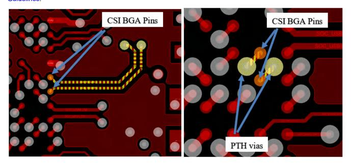
Figure 9-1. Serdes CSI Escapes for TOP layer (Left) and Inner layer (Right)
