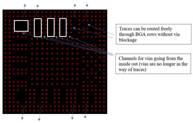
Figure 2-1. AM62Px BGA Array with Via Channels
