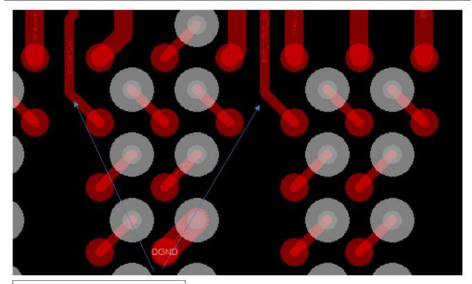
Traces can be routed freely through BGA rows without via blockage
