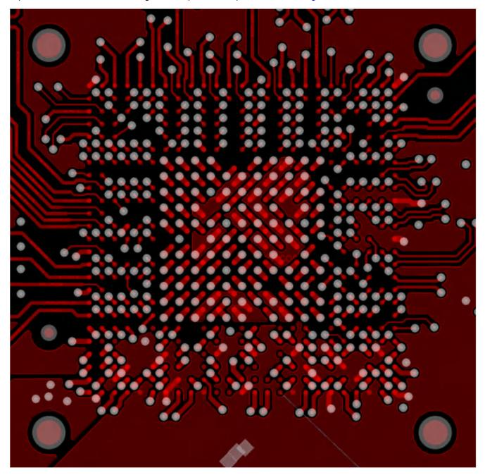
Figure 13-1. AM62Px with Complete Signal and Power Escapes
