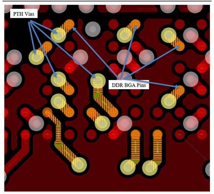
Figure 10-5. DDR Address/Cmd Escape
