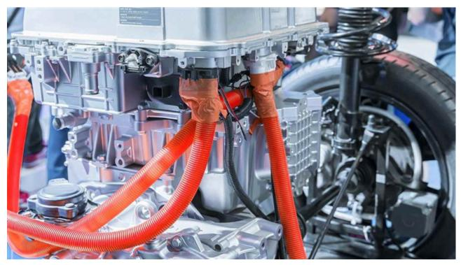
The electric vehicle (EV) traction inverter is the core of the EV. It converts DC from the high-voltage battery to multiphase (usually three-phase) AC to drive the traction motor, and also controls power regeneration from braking. EV electronics are shifting from 400-V to 800-V architectures, which promise:
