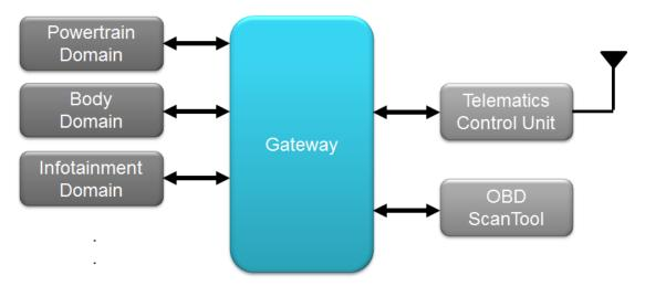
Figure 1. A Typical Vehicle Network Configuration Showing the Gateway
