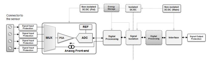
Figure 1. Temperature Transmitter Block Diagram
