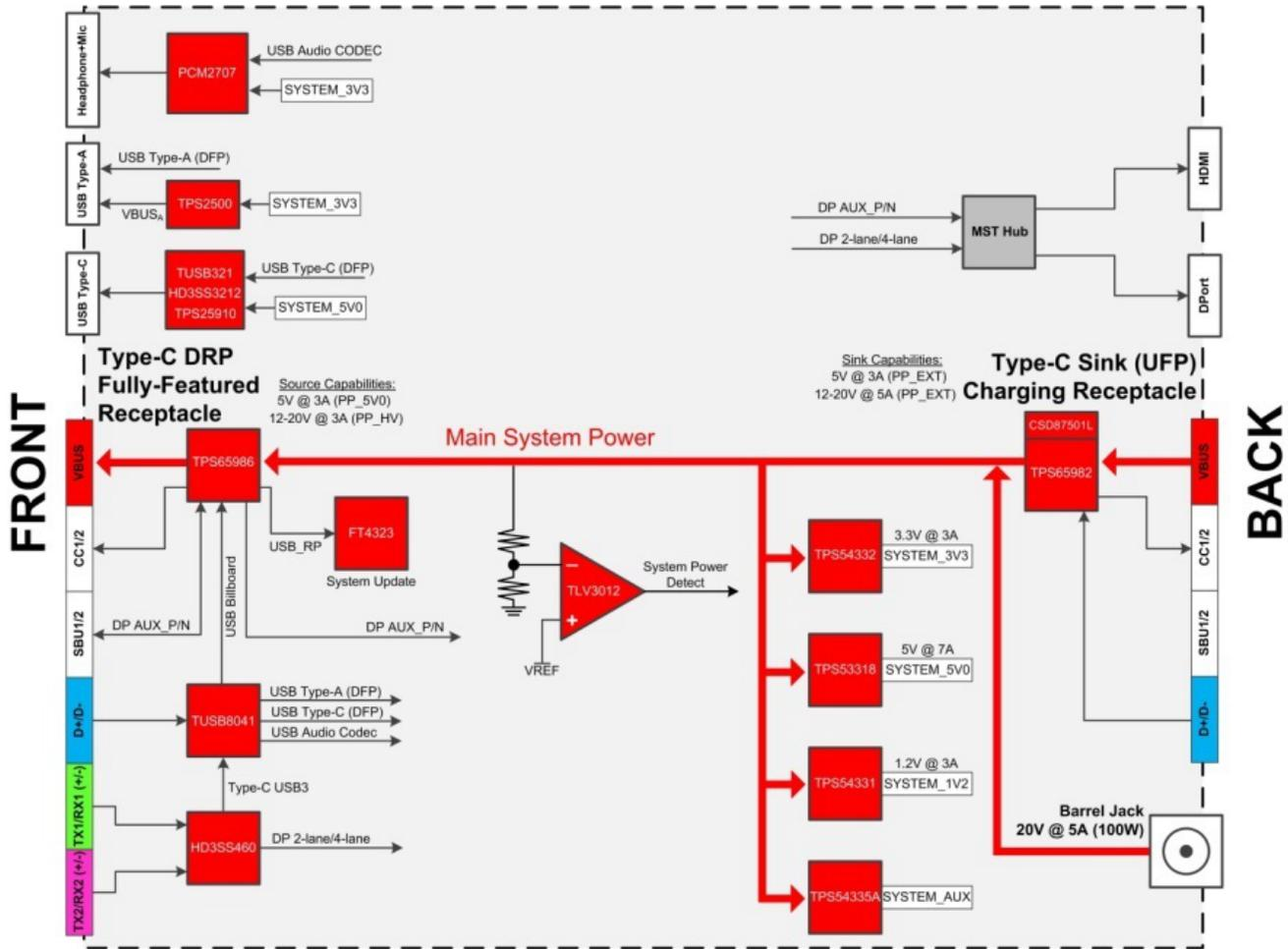
**Figure 2. Revised Minidock Block Diagram Based on Physical Location of ICs**
