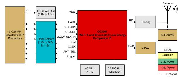
Figure 1-1. BP-CC3301 Block Diagram
