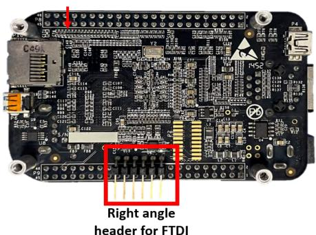
Figure 3-6. Bottom View of Modified BBB
