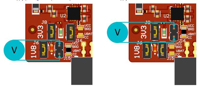
Figure 2-7. Active Current Measurement
