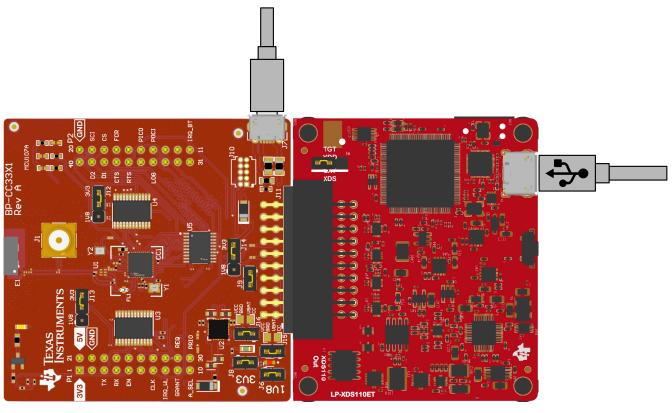
Figure 3-7. BP-CC3301 Connected to LP-XDS110 (ET)
