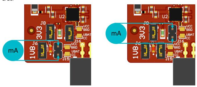
Figure 2-6. Low Current Measurement
