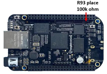
Figure 3-5. Top View of Modified BBB
