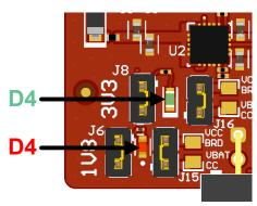
Figure 2-2. LEDs D4 & D5
