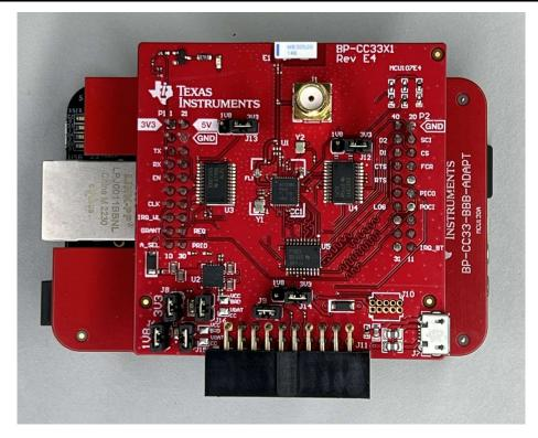
Figure 3-4. BP-CC3301 + BBB with Adapter Board
