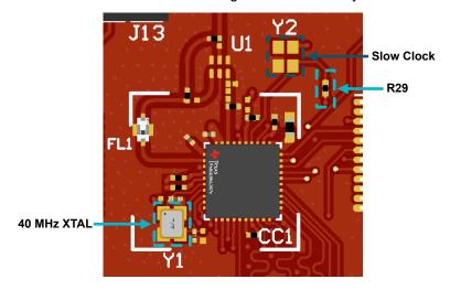
Figure 2-8. BP-CC3301 Clock Circuitry
