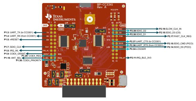
Figure 2-3. BP-CC3301 BoosterPack Header Pinout
