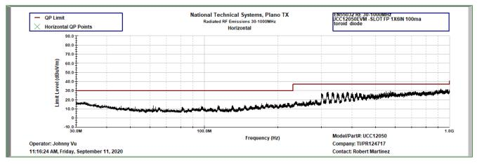
Figure 8-3. Horizontal, Ferrite Beads L1, L2, -5.15 dB (920 MHz), 100 % Load (500 mW)
