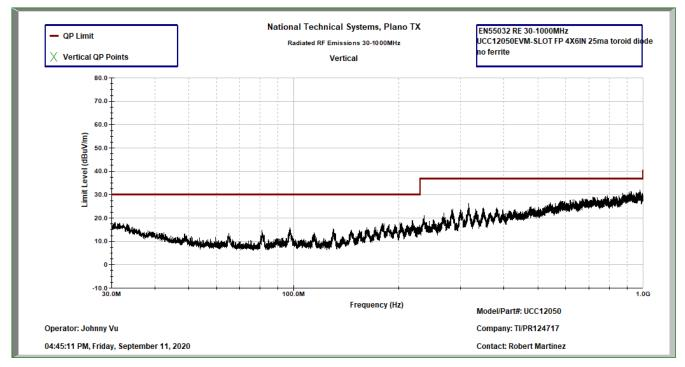
Figure 8-8. Vertical, no Ferrite Beads, -4.83 dB (980 MHz), 25% Load (125 mW)
