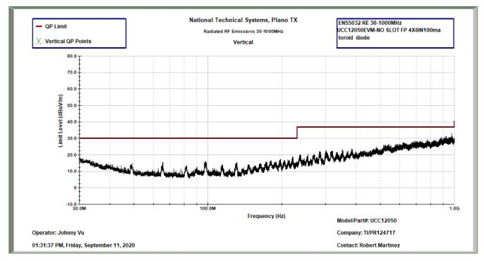
Figure 8-6. Vertical, Ferrite Beads L1-L8, -3.97 dB (975 MHz), 100% Load (500 mW)
