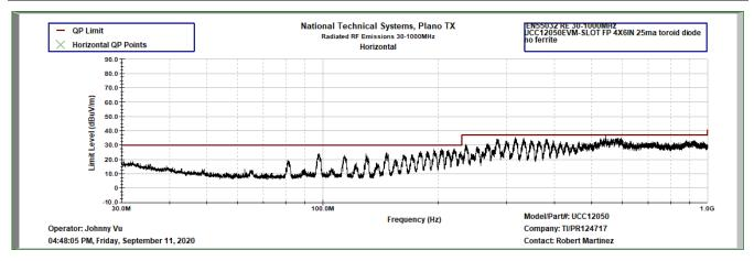
Figure 8-7. Horizontal, no Ferrite Beads, -0.11 dB (544 MHz), 25% Load (125 mW)
