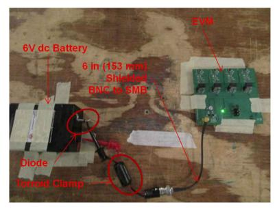
Figure 8-2. CISPR 32 V<sub>INP</sub> Battery to EVM Test Setup
