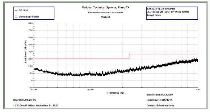
Figure 8-4. Vertical, Ferrite Beads L1, L2, -5.38 dB (930 MHz), 100 % Load (500 mW)
