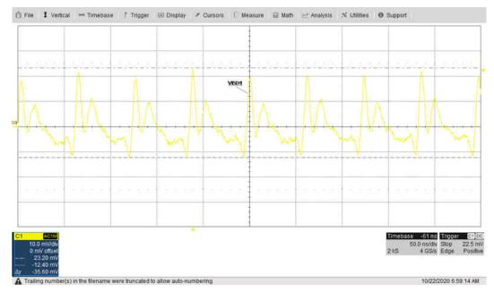
Figure 6-2. V<sub>ISO1</sub> (5 V) High Frequency, AC Ripple Voltage About 35 mV, 16 MHz
