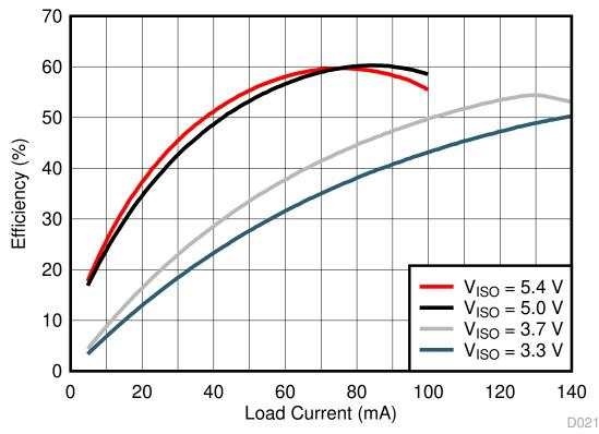
Figure 3-1. 5-V Input Typical Efficiency vs Load, V<sub>INP</sub> = 5.0 V, T<sub>A</sub> = 25°C, (UCC12050 Data Sheet, Page 1)
