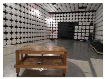
Figure 8-1. Anechoic Chamber – CISPR 32 Radiated EMI Test
