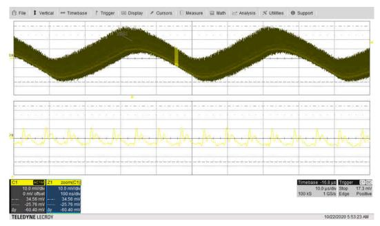
Figure 6-1. V<sub>ISO1</sub> (5 V) Modulated AC Ripple Voltage About 60 mV, 25 kHz
