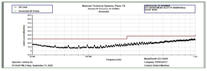
Figure 8-5. Horizontal, Ferrite Beads L1-L8, -5.06 dB (975 MHz), 100% Load (500 mW)
