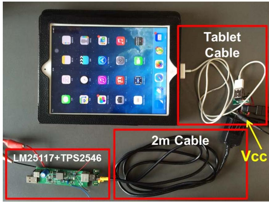
Figure 15 USB device charging test set-up
