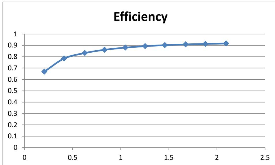
Figure 1 Efficiency versus load current (in Amps)
