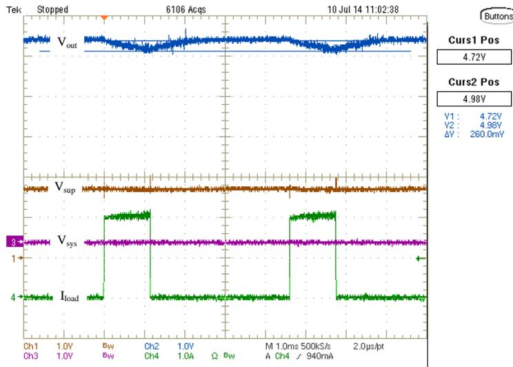
Figure 13:  $V_{out}$  Load Transient when  $V_{sup} = 1.7V$
