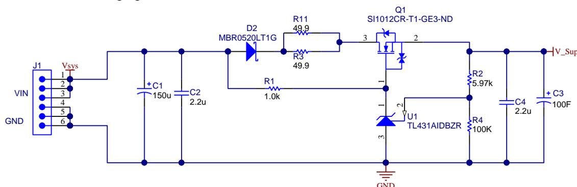
**Figure 3: Supercap Charger Circuit**
