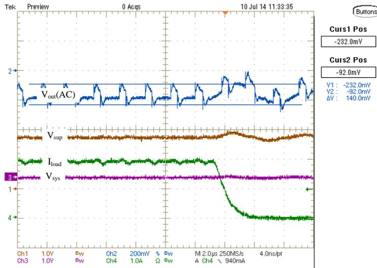
Figure 14:  $V_{out}$  Switching Ripple at  $V_{sup} = 1.7V$
