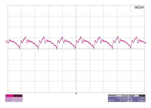
The 16V output ripple voltage (AC coupled) is shown below. The image was taken with the 16V output loaded to 6A, the 28V output loaded to 7A, and the input voltage set to 51V. (50mV/DIV, 5uS/DIV)
