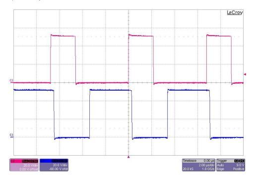
The photo below shows both the 16V and 28V switching voltage nodes. The image was taken with the 16V output loaded to 6A, the 28V output loaded to 7A, and the input voltage set to 51V. (20V/DIV, 2uS/DIV)
