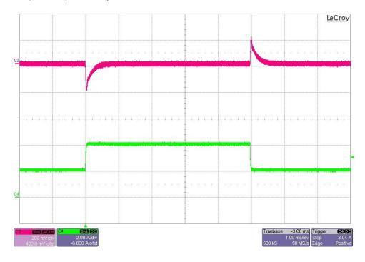
The photo below shows the 28V output voltage (ac coupled) when the load current is stepped between 2A and 7A. The 16V output was loaded to 4A and the input voltage was set to Vin = 48V. (500mV/DIV, 2A/DIV, 1mS/DIV)
