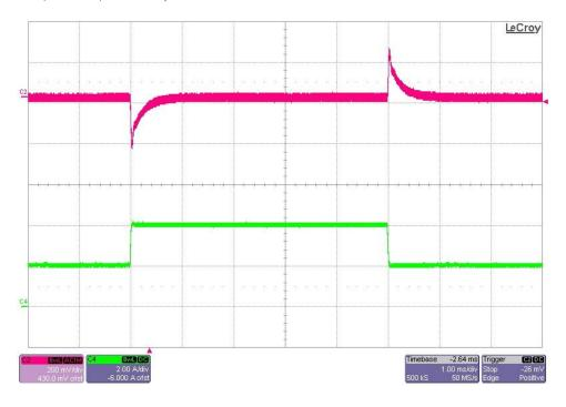
The photo below shows the 16V output voltage (ac coupled) when the load current is stepped between 2A and 6A. The 28V output was loaded to 2A and the input voltage was set to Vin = 48V. (500mV/DIV, 2A/DIV, 1mS/DIV)
