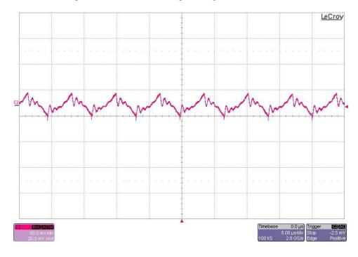
The 28V output ripple voltage (AC coupled) is shown below. The image was taken with the 16V output loaded to 6A, the 28V output loaded to 7A, and the input voltage set to 51V. (50mV/DIV, 5uS/DIV)
