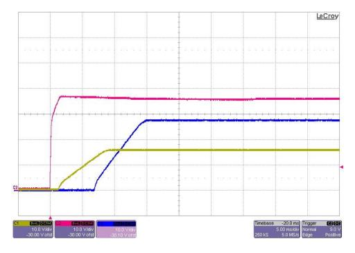
The photo below shows the output voltage startup waveform after the application of 51V in. The 16V and 28V outputs were loaded to 0A. (10V/DIV, 5mS/DIV)
