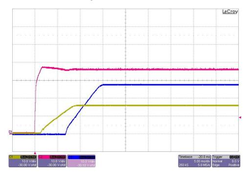
The photo below shows the output voltage startup waveform after the application of 51V in. The 16V output was loaded to 4A and the 28V output was loaded to 2A. (10V/DIV, 5mS/DIV)
