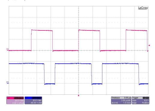
The photo below shows both the 16V and 28V switching voltage nodes. The image was taken with the 16V output loaded to 6A, the 28V output loaded to 7A, and the input voltage set to 36V. (20V/DIV, 2uS/DIV)
