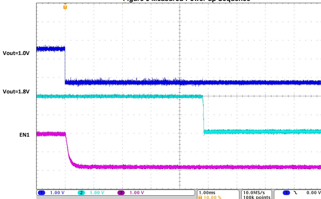
**Figure 6 Measured Power down Sequence**
