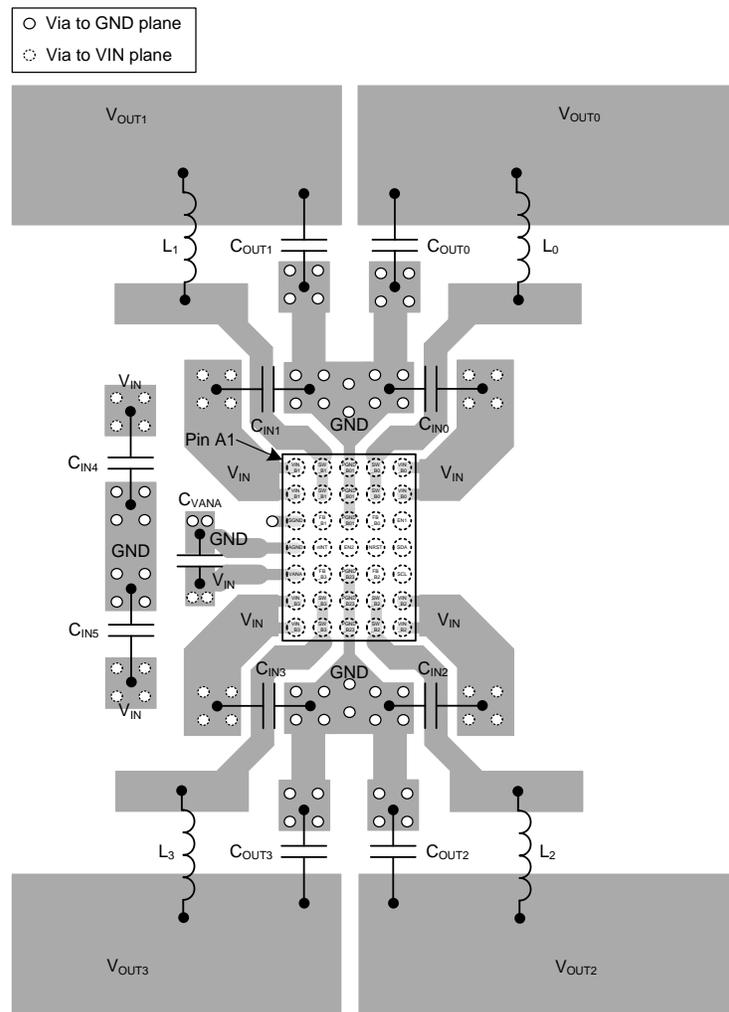
**Figure 3: PCB layout example for LP8758-E0**
