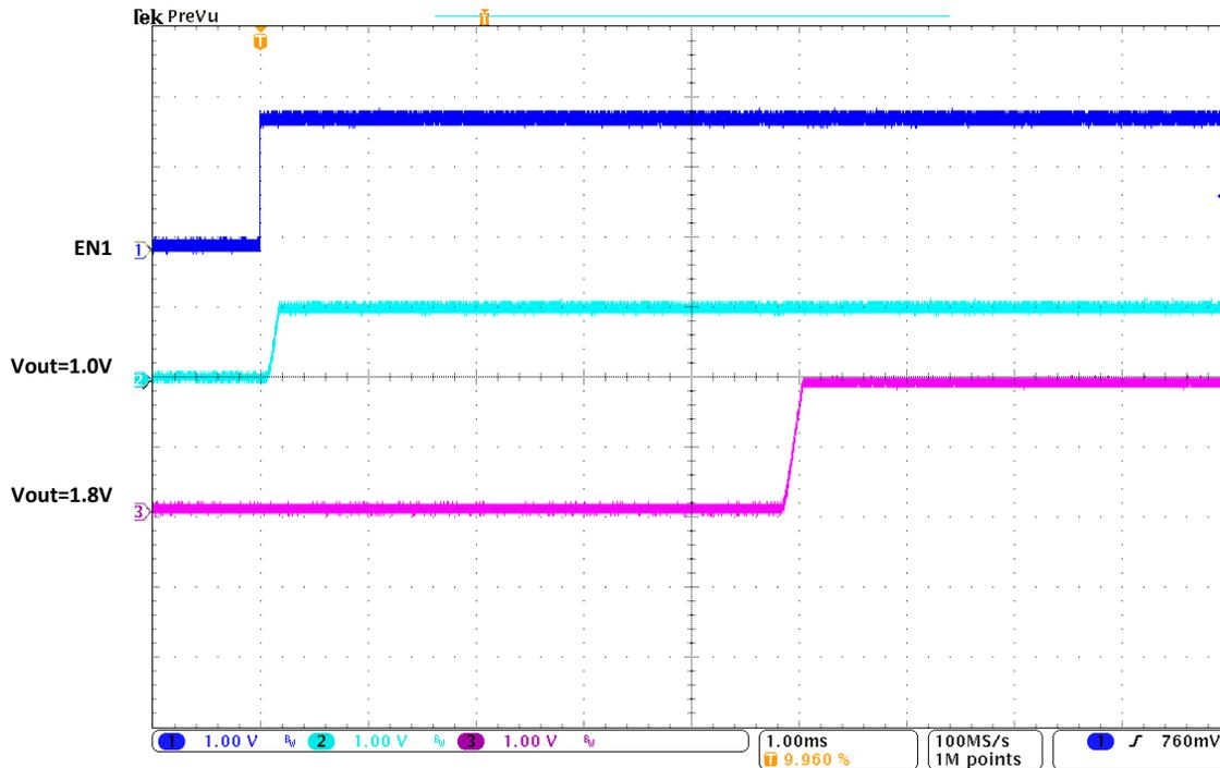
**Figure 5 Measured Power up Sequence**
