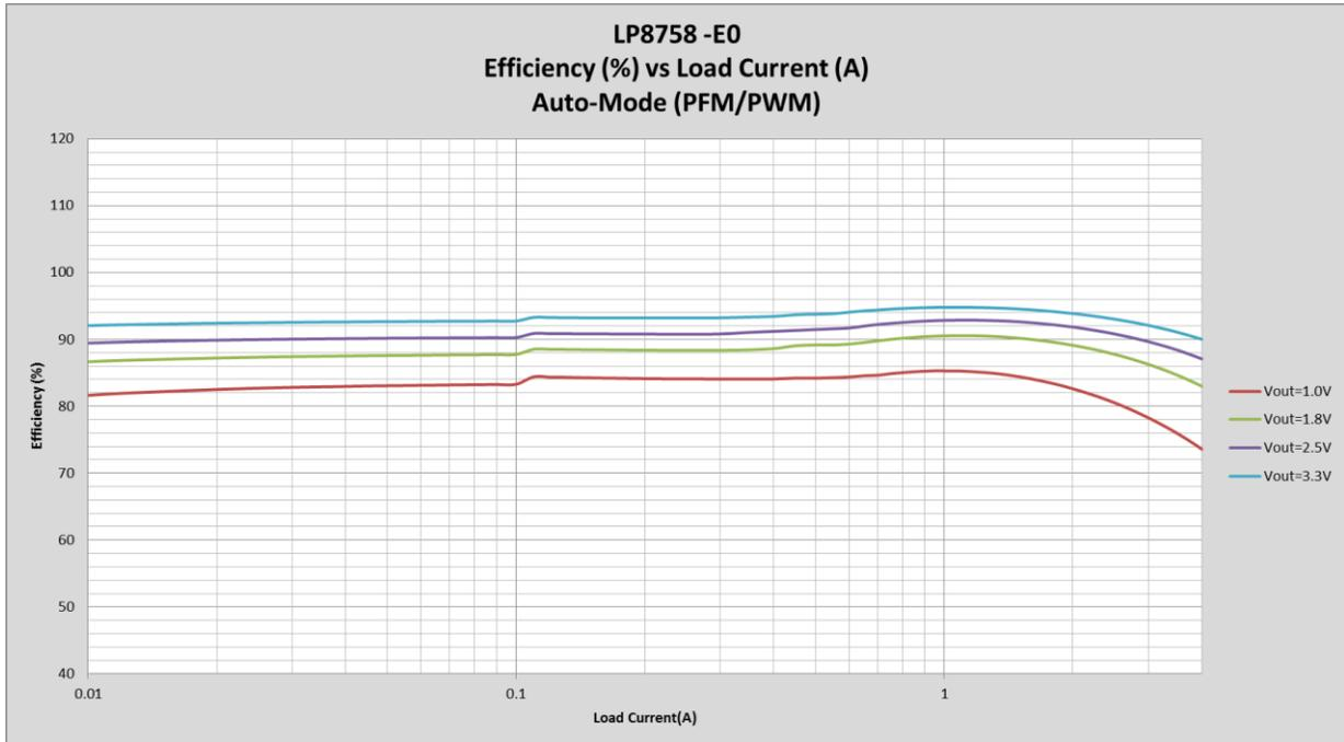
**Figure 4: Output Voltage Efficiency in Auto Mode**
