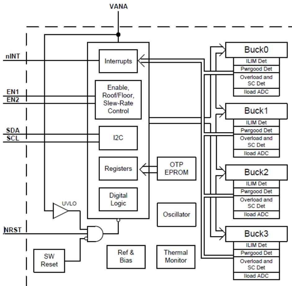
Figure 2: LP8758 Functional Block Diagram
