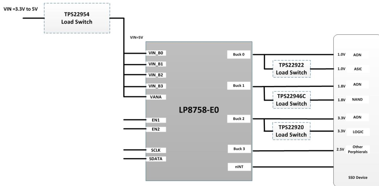
Figure 1 Comprehensive block diagram
