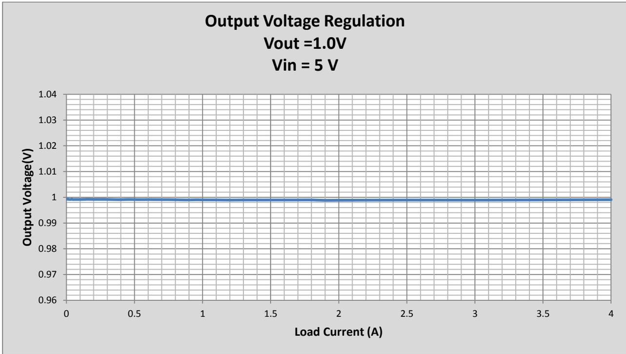
**Figure 7 Output voltage vs Load Current**
