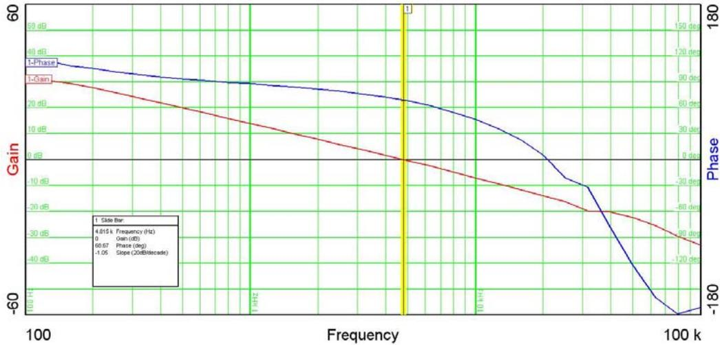
The figure below is the loop gain of the converter with a 24V input and a 1.1A load. The Bandwidth is 2.6 KHz, the Phase Margin is 74 degrees, and the Gain Margin is 16 dB.
