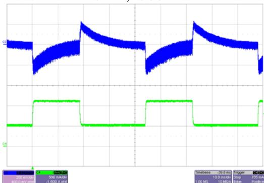
Output load step, 0.55A to 1.1A, 24Vin
