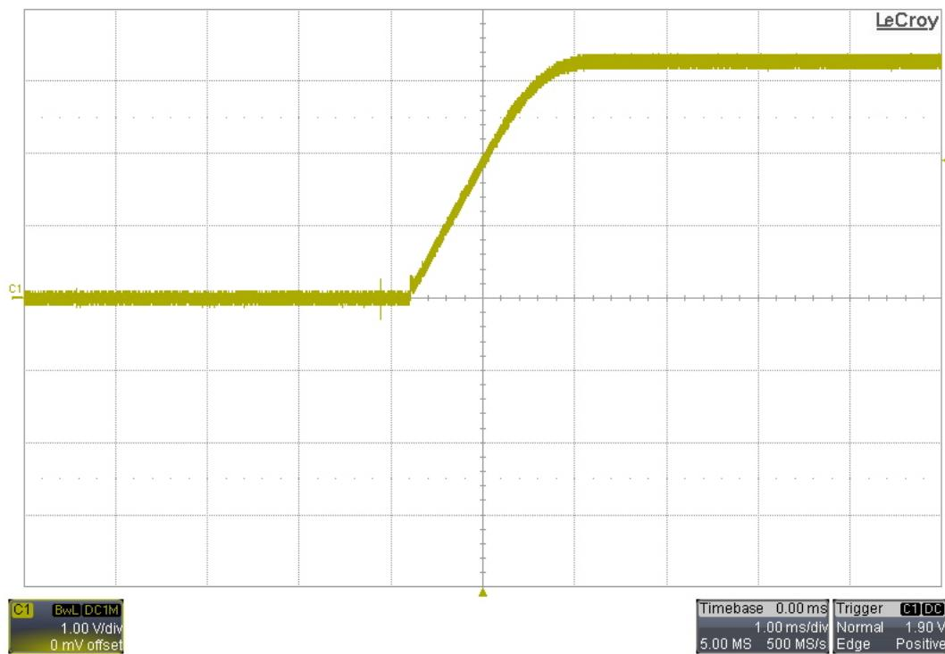
**7.5 2.5V Buck; 5V Input – No Load**
