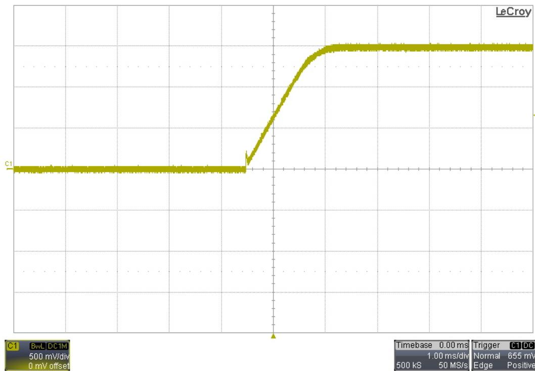
**7.9 1.0V Buck; 5V Input – No Load**
