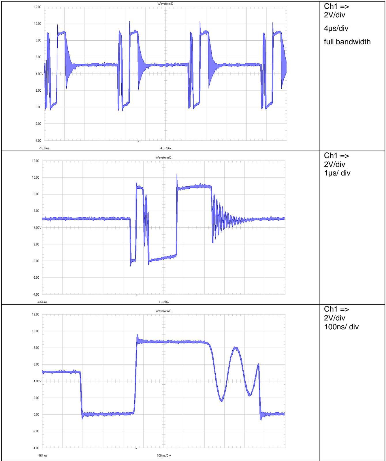
**Figure 26 – the SEPIC itself runs in discontinuous mode DCM**
