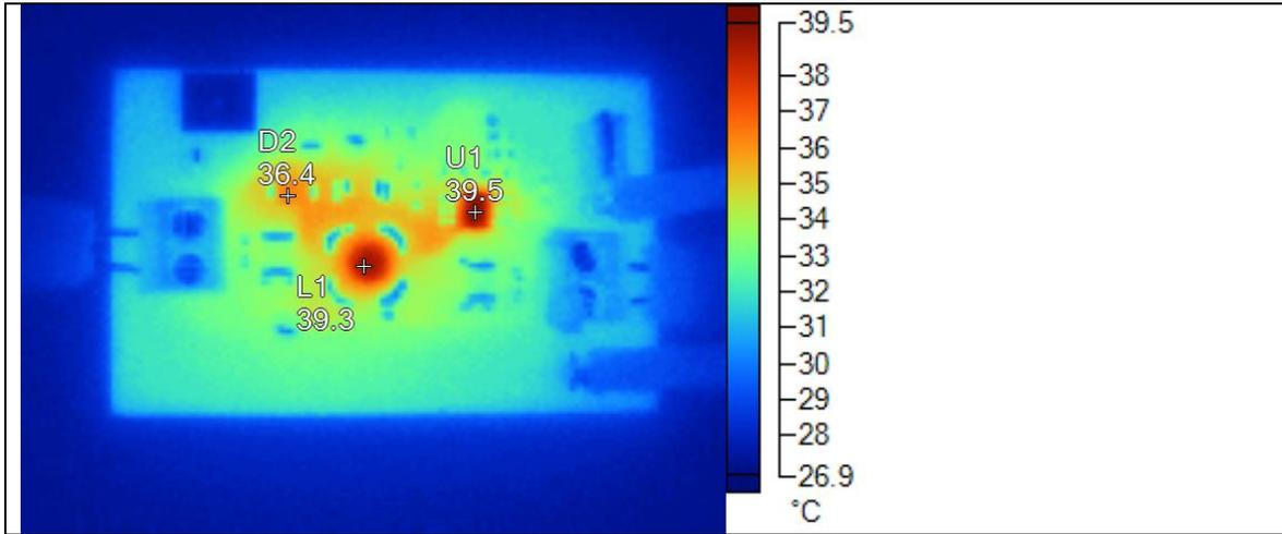
**Figure 28 – the temperature rise is below 20K**
