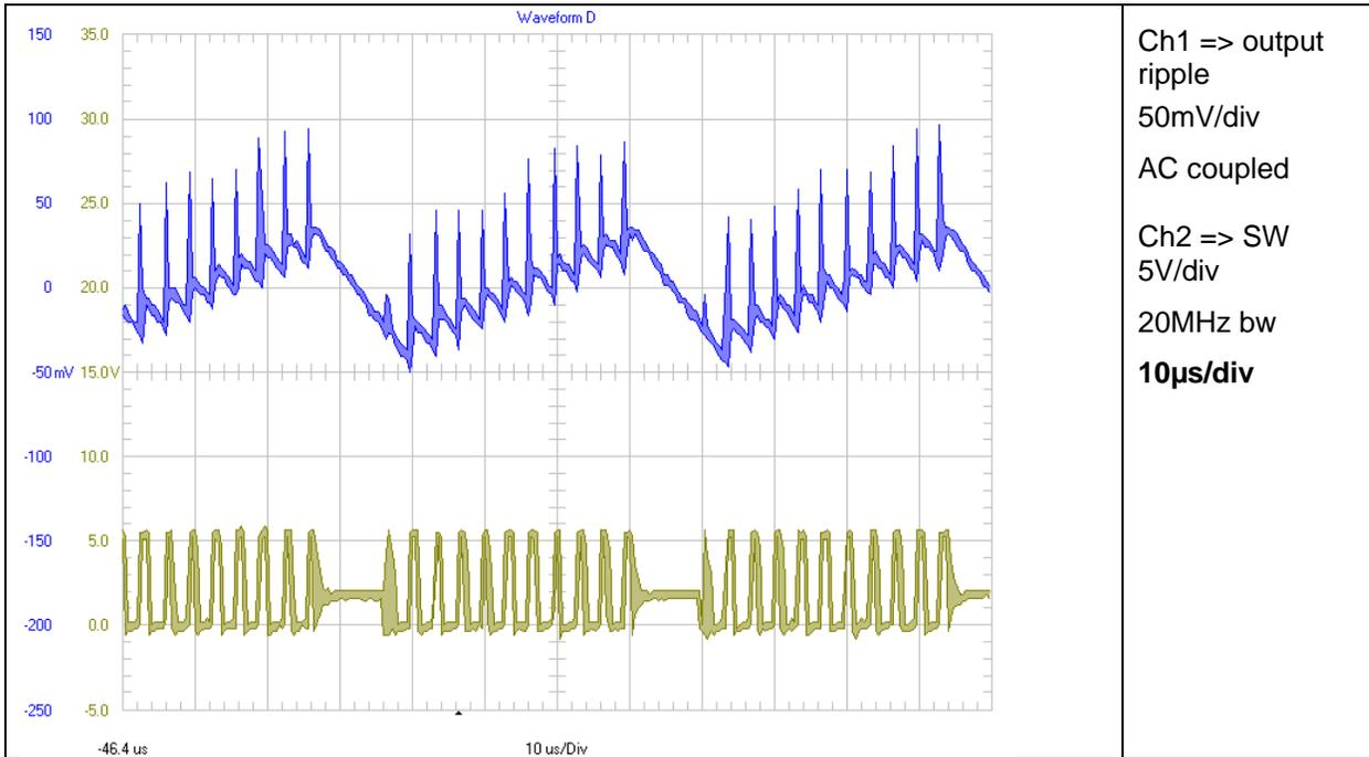
**Figure 12 – the hysteretic mode could be seen here**
