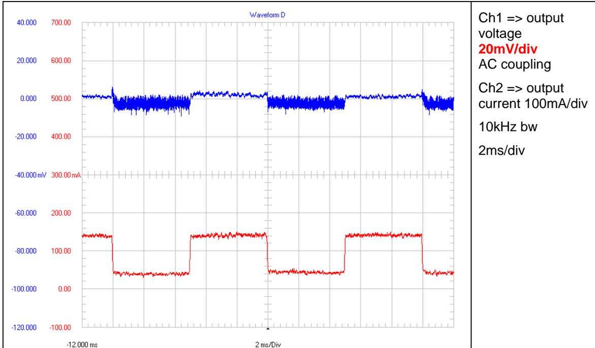
**Figure 19 – the OPEN LOOP control architecture provides fine transient response**
