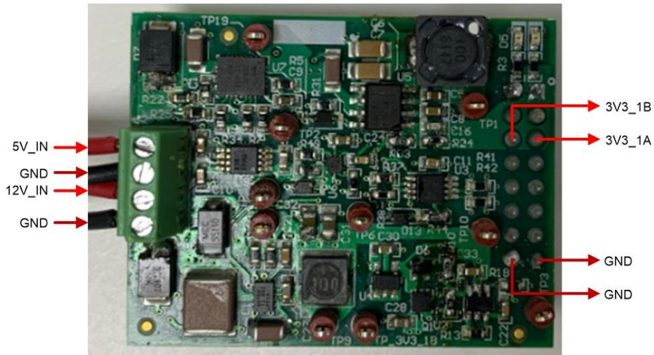
The TIDA-010052 board is very compact, with 45.00-mm x 35.00-mm dimensions. J2 is a 4-pin connector, which supplies 5-V and 12-V input voltages. J1 is the output connector, giving a 3.3-V power supply for external use respectively.
