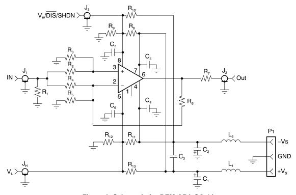
Figure 2. Schematic for DEM-OPA-SO-1A
