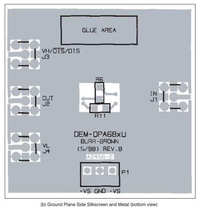
Figure 3. DEM-OPA-SO-1A Demonstration Board Layout
