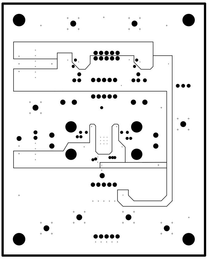
Figure 3. VCA2615EVM PCB Power Layer (Top View)
