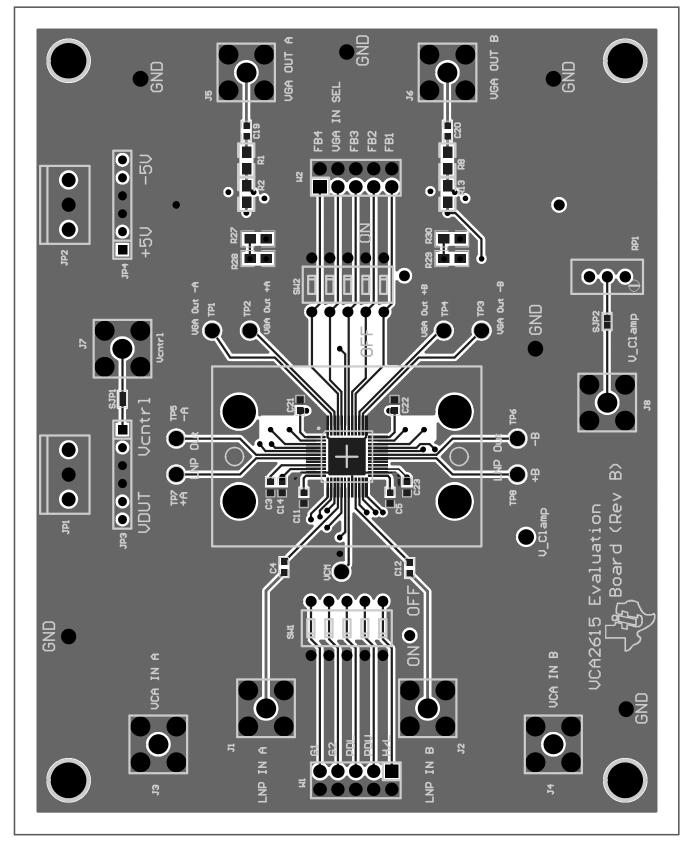
Figure 2. VCA2615EVM PCB Top Layer (Top View)
