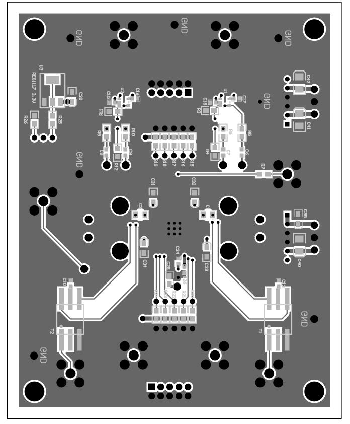
Figure 5. VCA2615EVM PCB Bottom Layer (Bottom View)
