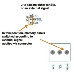
Figure 9. BUF22821EVM Jumper JP2 Set for External Signal Switching
