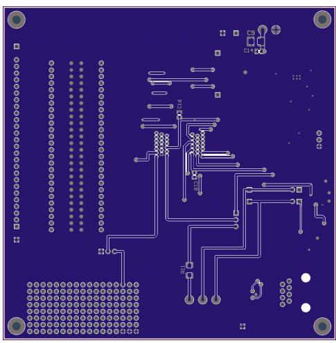
Figure 25. BUF22821EVM PCB Bottom Layer (Solder Side)
