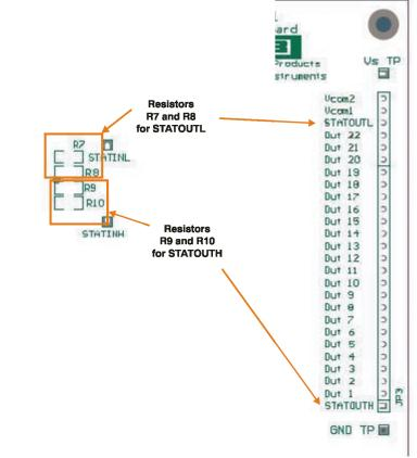
Note: Resistors R7 through R10 are installed at the factory.
