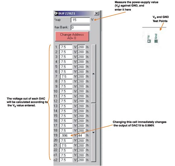
Figure 12. Power Supply Measurement and Recording
