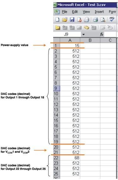
Figure 15. Working with a Saved BUF22821 Data File
