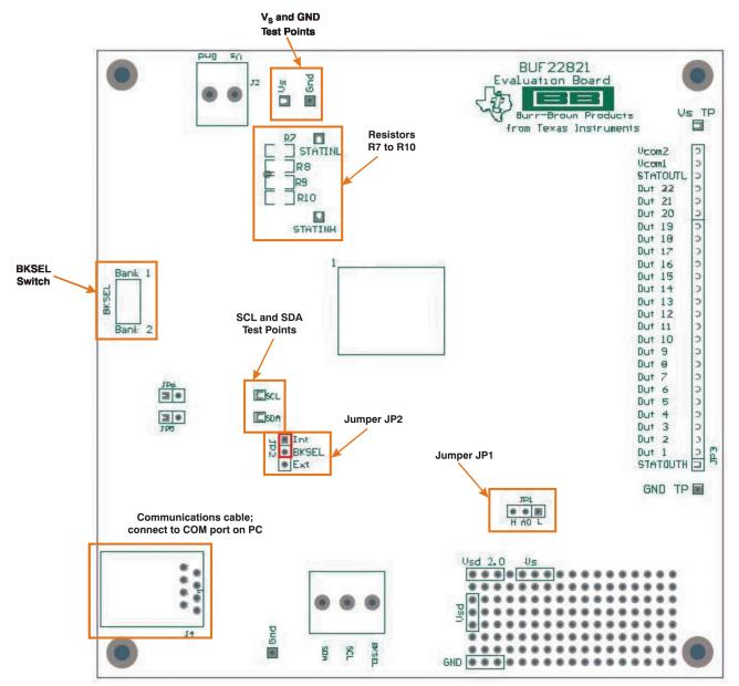
Figure 4. BUF22821EVM Switch and Jumper Locations
