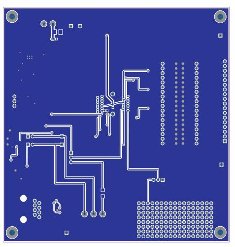
Figure 24. BUF16821EVM PCB Bottom Layer (Solder Side)
