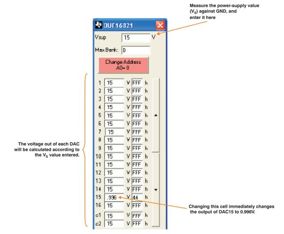
Figure 11. Power Supply Measurement and Recording
