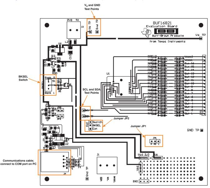
Figure 4. BUF16821EVM Switch and Jumper Locations
