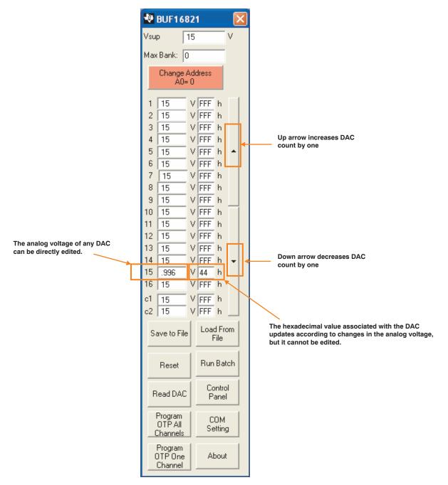
Figure 16. Changing the DAC Analog Voltage
