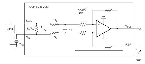
Figure 2. Measurement with Shunt
