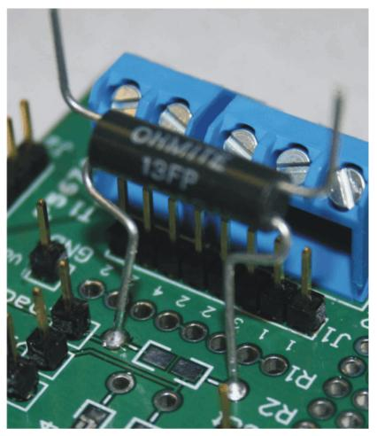
Figure 8. Radial Package in R2
