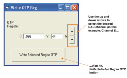
Figure 20. Program OTP Out Button and Write OTP Reg Dialog
