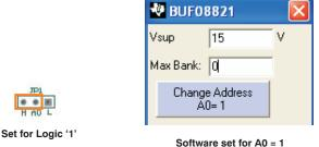
Figure 6. BUF08821EVM Jumper JP1 Set for Logic '1'
