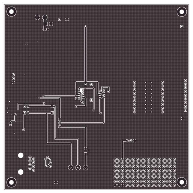
Figure 24. BUF08821EVM PCB Bottom Layer (Solder Side)
