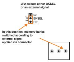
Figure 9. BUF08821EVM Jumper JP2 Set for External Signal Switching
