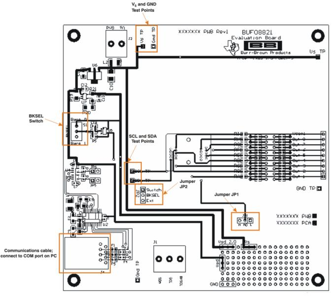
Figure 4. BUF08821EVM Switch and Jumper Locations
