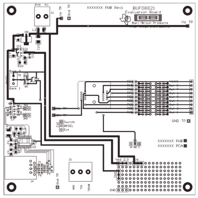
Figure 23. BUF08821EVM PCB Top Layer (Component Side)
