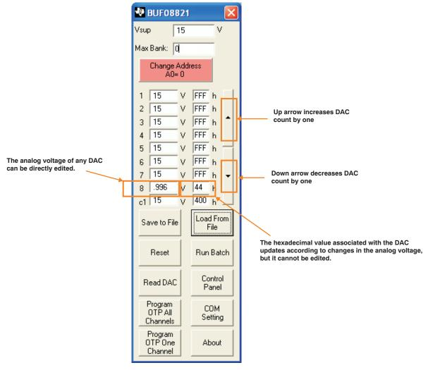
Figure 16. Changing the DAC Analog Voltage
