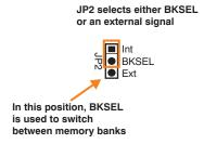
Figure 8. BUF08821EVM Jumper JP2 Set for BKSEL Switching
