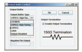
Figure 9. Output Buffer Config (each output)
