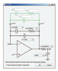
Figure 7. Loop Filter, Additional External Components
