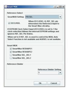
Figure 4. Smart MUX
