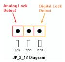
Figure 12. Lock Detect Select Jumper
