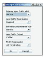
Figure 3. Input Buffer Properties
