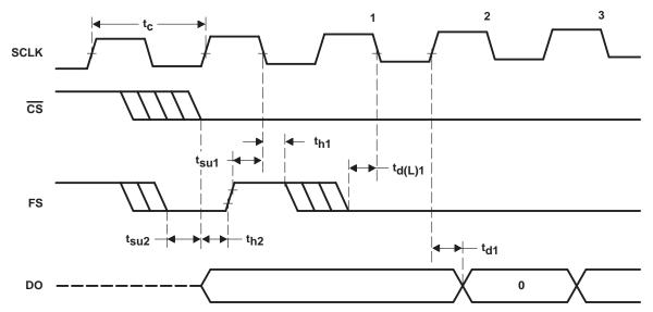
Figure 4–3. Microprocessor Interface Timing (Normal Sample Mode, INV CLK = Low)
