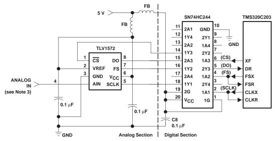
(a) Hardware Connection with Cabling Longer than 6 Inches to the DSP
