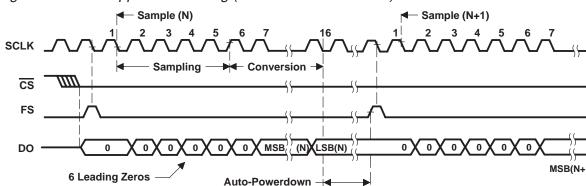
Figure 4–6. DSP Application Timing (Intermittent Conversion)
