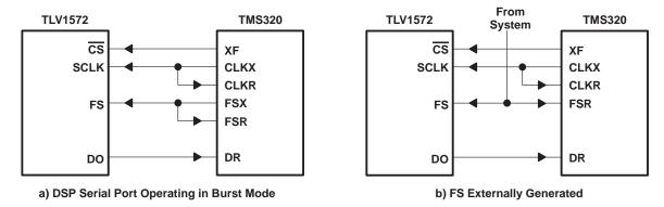
Figure 4-5. Typical Timing Diagram for DSP Application
