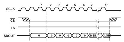
To use the TLV1572 in a non-DSP application, the FS input should be pulled high as shown in Figure 4–9.
