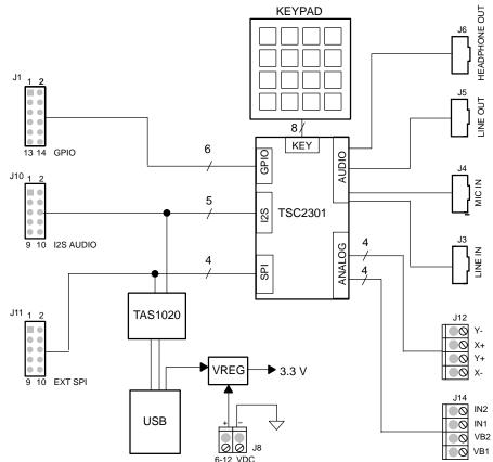
The digital control interface is through either the USB bus or an external SPI bus. The onboard microprocessor can be disabled, allowing the external SPI bus to control the TSC2301.
