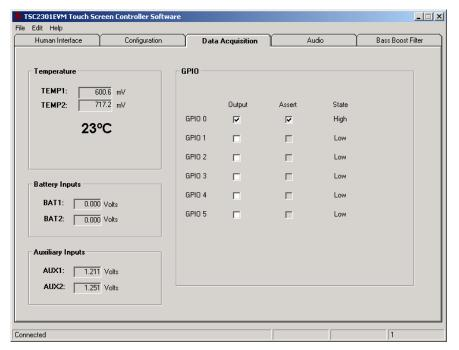
When on this screen, the TSC2301 is commanded to perform a PORT SCAN function, which updates the battery and auxiliary input voltage readings, and then is commanded to perform a TEMP1 and TEMP2 measurement. These measurements are all repeated once every second, and the results are displayed on this screen.
