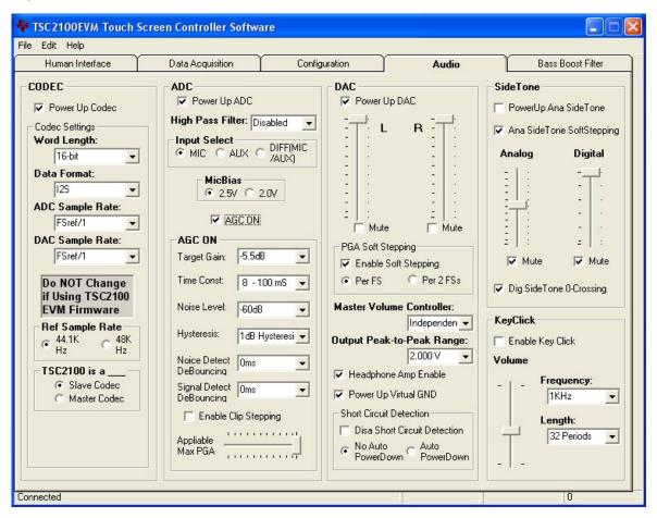
Figure 3–9. Audio Screen With AGC On
