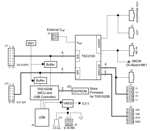
The digital control interface is through either the USB bus or an external SPI bus. The onboard microprocessor can be disabled, allowing the external SPI bus to control the TSC2100.
