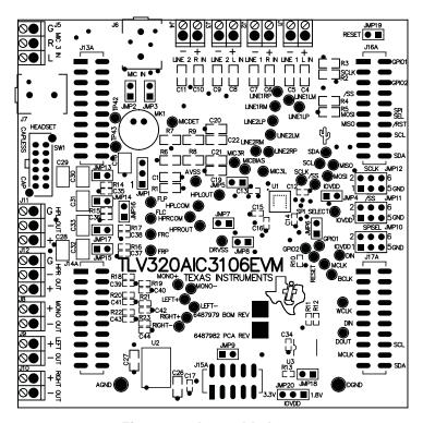
Figure 31. Assembly layer
