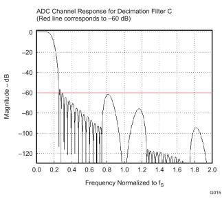
Figure 2-19. ADC Decimation Filter C, Frequency Response
