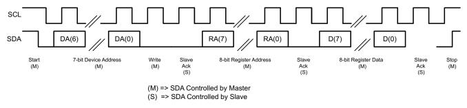
Figure 2-48. I<sup>2</sup>C Write
