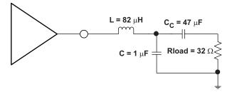
Figure 2-5. Configuration for Using Headphone Amplifier in Class-D Mode
