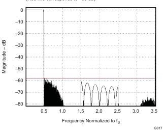
DAC Channel Response for Interpolation Filter B (Red line corresponds to -58 dB)
