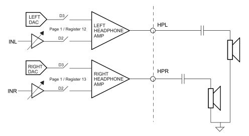
Figure 2-2. Stereo Headphone Configuration
