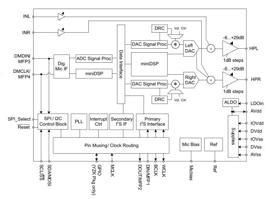
Figure 1-1. Simplified Block Diagram
