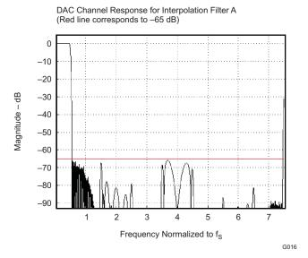
Figure 2-31. DAC Interpolation Filter A, Frequency Response
