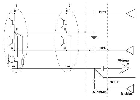
Figure 2-52. Jack Connections for Headset Detection
