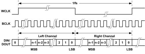
Figure 2-34. Timing Diagram for Right-Justified Mode
