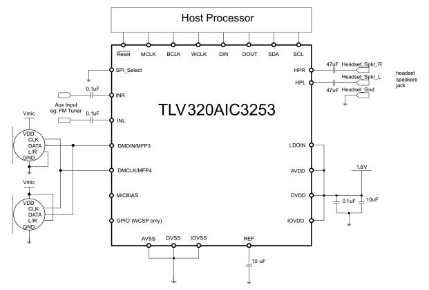
Figure 1-2. Typical Circuit Configuration
