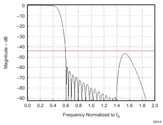
Figure 2-18. ADC Decimation Filter B, Frequency Response
