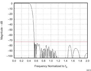
Figure 2-17. ADC Decimation Filter A, Frequency Response
