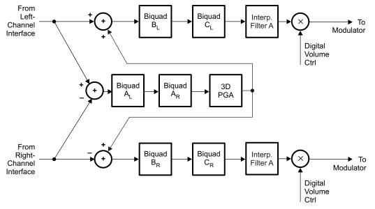
Figure 2-28. Signal Chain for PRB\_P23
