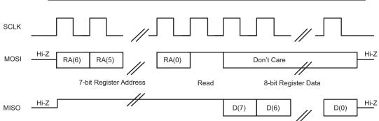
Figure 2-51. SPI Timing Diagram for Register Read
