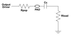
Figure 2-3. Conceptual Circuit for Pop-Free Power-up
