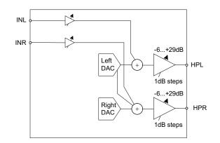
Figure 2-1. Low Power Analog Bypass
