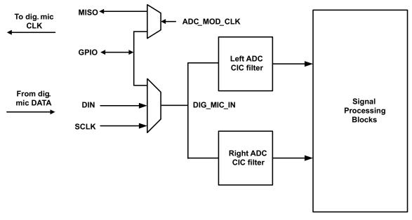
Figure 2-6. Digital Microphone in TLV320AIC3253
