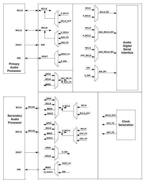
Figure 2-44. Audio Serial Interface Multiplexing
