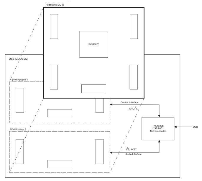
Figure 1. PCM3070EVM-K Block Diagram
