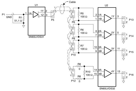
Termination resistors R5, R6, and R7 must be removed.
