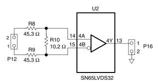
Figure 6-1. TIA/EIA-422 Data to an LVDS Receiver Schematic
