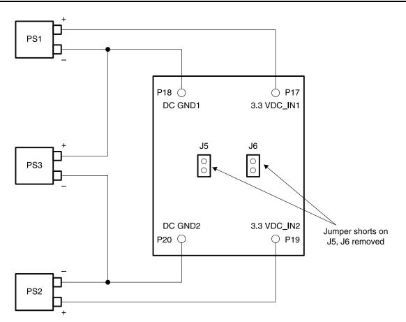
Figure 5-1. Test Setup
