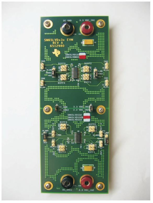
Figure 1-1. SN65LVDS31/32B EVM Printed-Circuit Board
