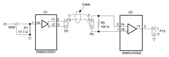
Figure 3-1. Point-to-Point Schematic Diagram
