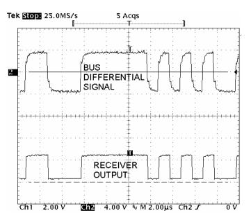
In this example, the oscilloscope cursors are used to indicate the 20-V offset that has been induced between the driver on one EVM and the receiver on another. This demonstrates the performance of the SN65HVD22 with offsets exceeding the capabilities of standard transceivers.
