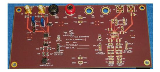
Note that the EVM printed circuit board includes a location (U1) for a full-duplex transceiver. This allows for future EVM configurations using the same board.
