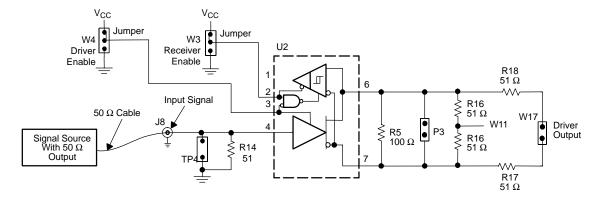
The input/output characteristics of the driver can be observed by probing TP4 (driver input) and either P3 or W17 (driver output). In addition to the single-ended outputs (with respect to GND2) and the differential outputs available at P3 and W17, the common-mode output can be observed using W11 as a test point.
