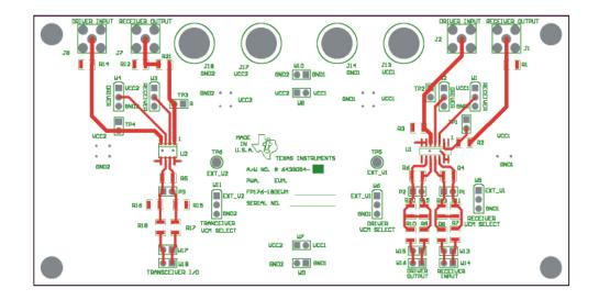
Figure 3-3. PWB Layer 2 (Split Ground Planes)
