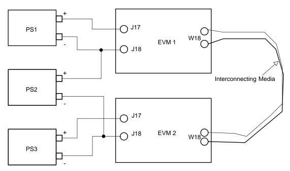
Power supply PS1 supplies the V<sub>CC2</sub> voltage to EVM1, and power supply PS3 supplies the V<sub>CC2</sub> voltage to EVM2. Power supply PS2 forces an offset between the ground reference of PS1 and PS3. Special care must be taken to make sure the grounds of the two EVMs are not connected together through instrumentation or non-isolated power supply earth ground or chassis connections. When using more than one probe with this test set up, make only one return connection to the oscilloscope.
