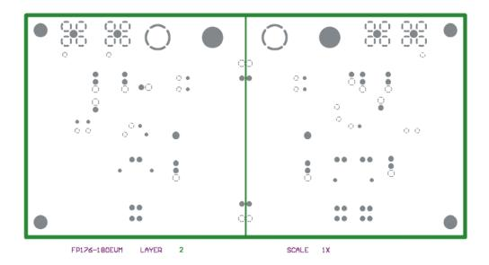
Figure 3-4. PWB Layer 3 (Split Power Planes)
