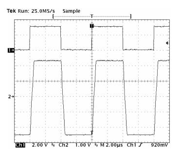
The effect of the driver slew rate limit is also evident when using the EVM in this configuration. The slope of the driver transitions is controlled to reduce high frequency content, which may create problems in long cable applications. The slew-rate control is designed for signaling rates up to 500 kbps in the SN65HVD22.
